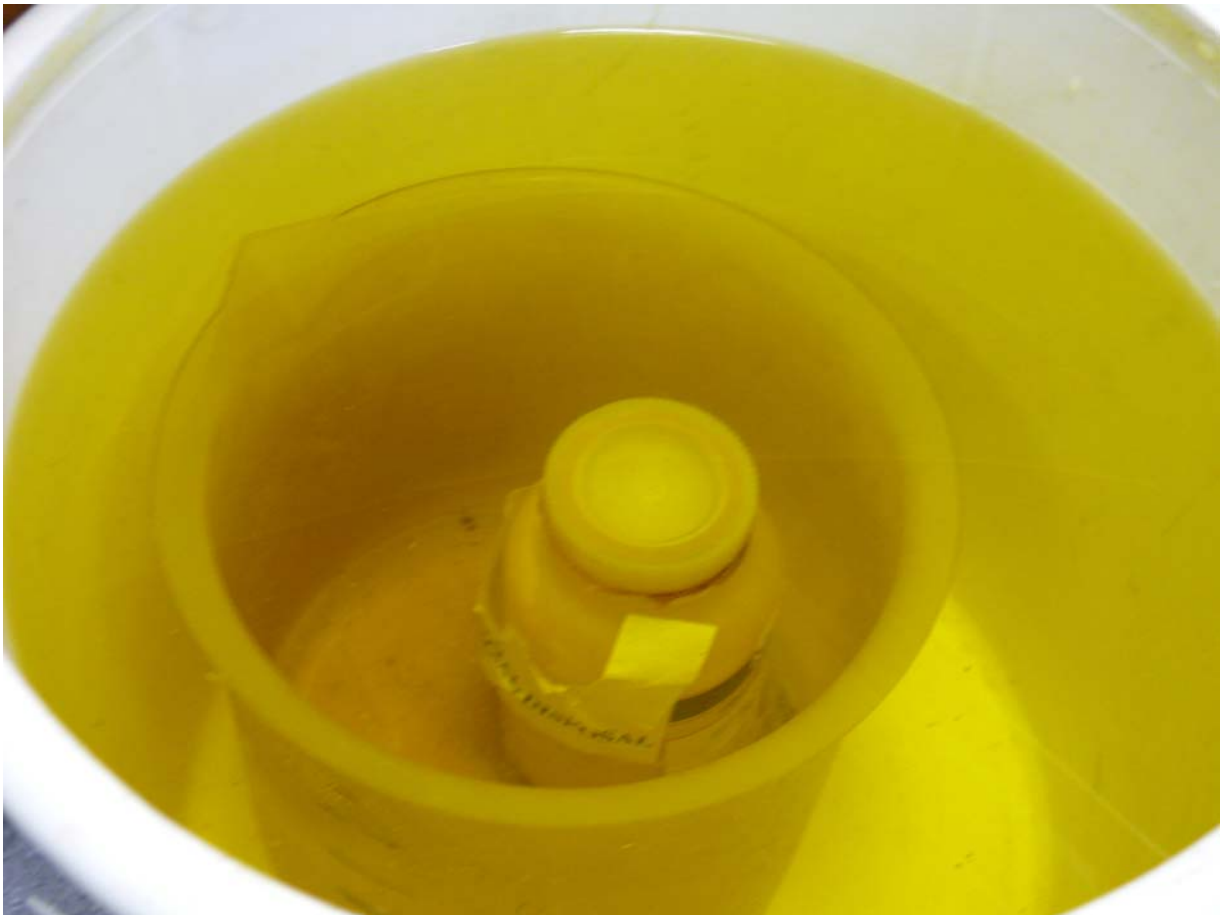
Image 1 – Plastic jar of picric acid submerged in bucket of water following rehydration.
