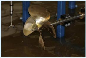
This new facility consists of a 4 m by 7 m, 1.4 m deep basin in which a model of the port infrastructure (often with a mobile bed included) and erosion protection solutions can be installed and tested. The basin is equipped with four submersible frequency-controlled power motor units and various sized propellers, which can simulate a wide range of vessel types.
