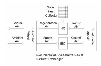
Figure 1: Schematic diagram of a desiccant-IEC air conditioning system
