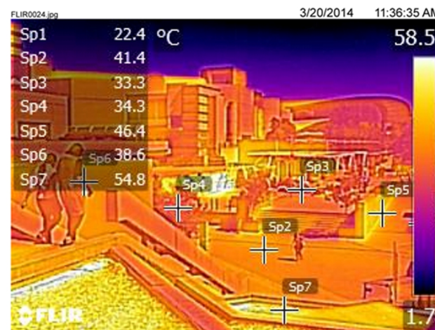
Figure 1: Hard urban surfaces such as asphalt, concrete and paving store heat in their thermal mass and make the public space a dangerous place to attend during heat stress (Riverbank Plaza, Adelaide, FLIR 6 thermal image taken by E. Sharifi).
