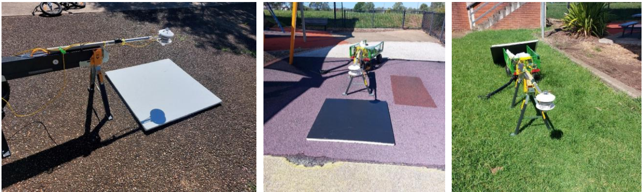
Figure 21. Albedo measurements with the albedometer at 0.50 m over the white mask (left), the black mask (centre), and without masks (right), as shown over different surfaces to demonstrate the method's application over various patches.
