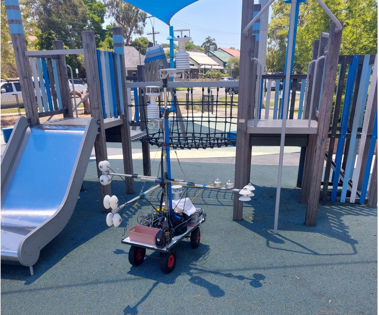
Figure 15. New version of the MaRTy mobile biometeorological instrument platform, including weather stations, net radiometers and UV radiometers.
