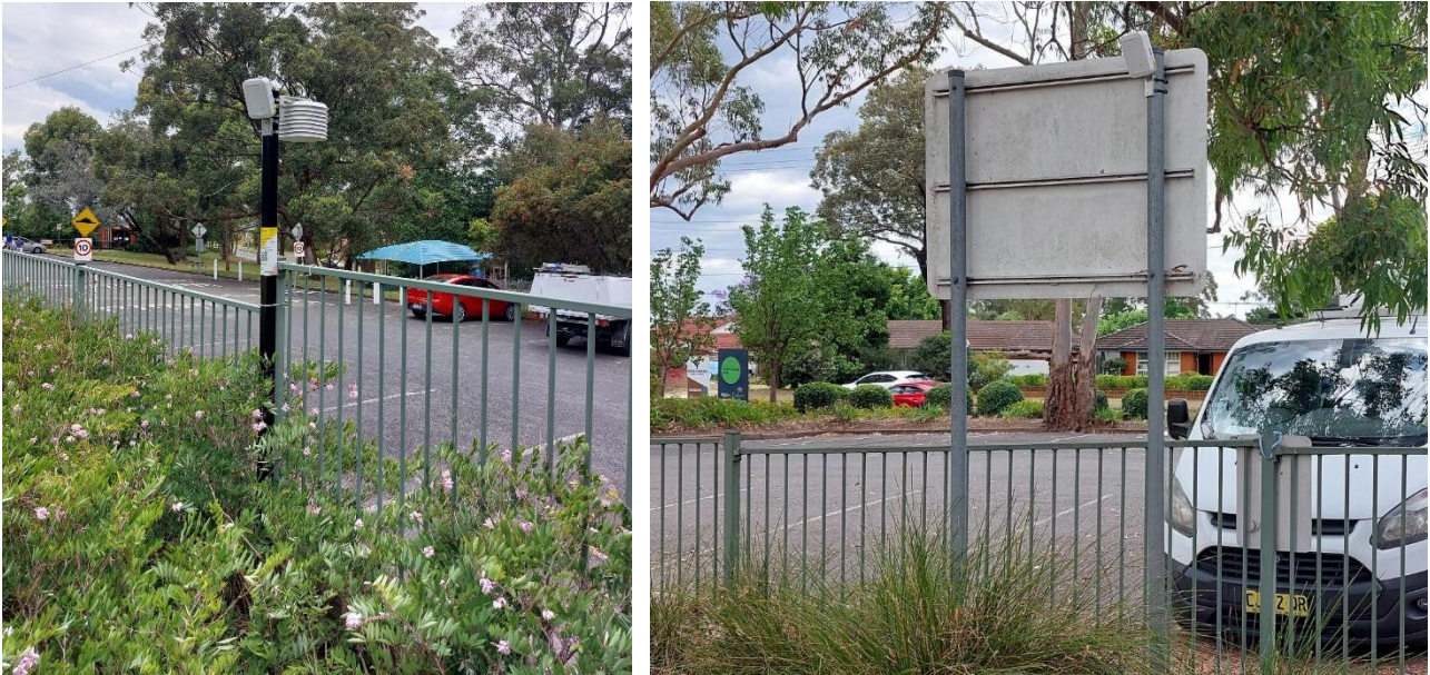
Figure 12. Equipment-facing people counters installed on a pole fastened to the fence near the swings (left) and on a sign pole near the carpark (right).
