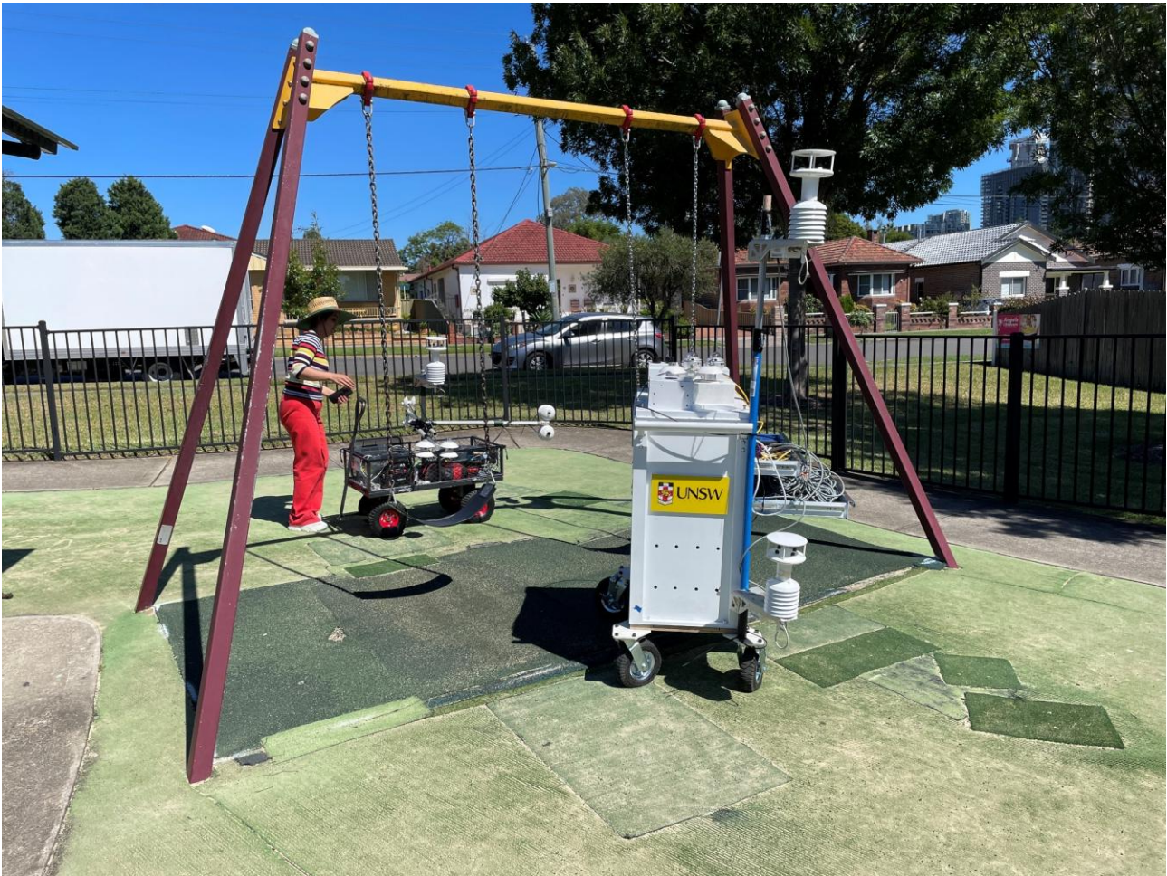
Figure 14. Mobile experimental setup used to record data along transects and characterise the local thermal comfort conditions and incoming solar and ultraviolet radiation. On the left, MaRTy, a mobile biometeorological instrument platform capable of measuring air temperature, humidity, wind speed and direction, GPS coordinates and mean radiant temperature using data captured in six directions by six solar and six infrared radiometers. These parameters are used to compute the local thermal comfort conditions, simulating the way the human body experiences heat. On the right, a cart equipped with solar and UV radiometers, as well as two weather stations at 0.3 m and 1.8 m from the ground.
