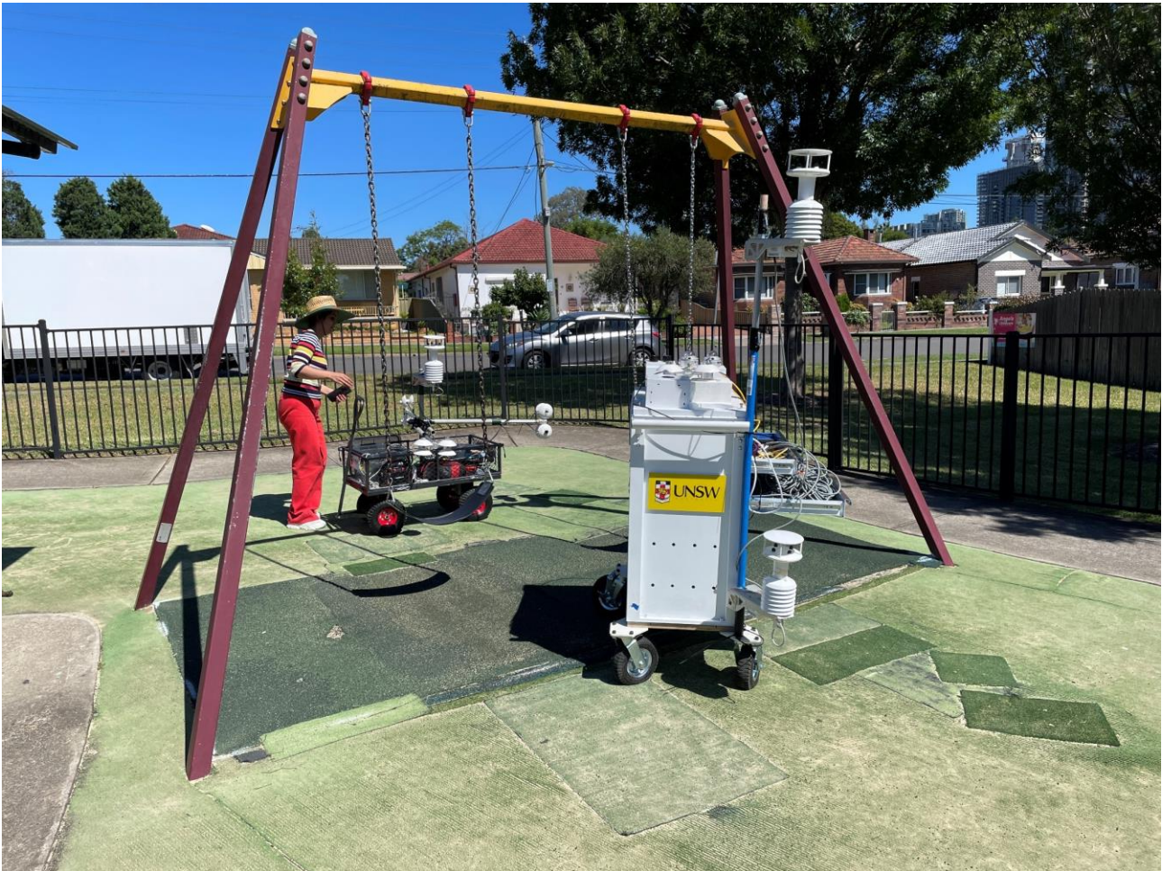
Figure 8. Mobile experimental setup used to perform transects and characterise the local thermal comfort conditions and incoming solar and ultraviolet radiation. On the left, MaRTy, a mobile biometeorological instrument platform capable of measuring air temperature, humidity, wind speed and direction, GPS coordinates and mean radiant temperature using data captured in six directions by six solar and six infrared radiometers. These parameters are used to compute the local thermal comfort conditions, simulating the way the human body experiences heat. On the right, a cart equipped with solar and UV radiometers, as well as two weather stations at 0.3 m and 1.8 m from the ground.
