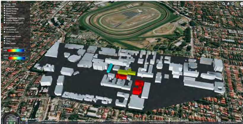
CityGML LOD1 and energy consumption
