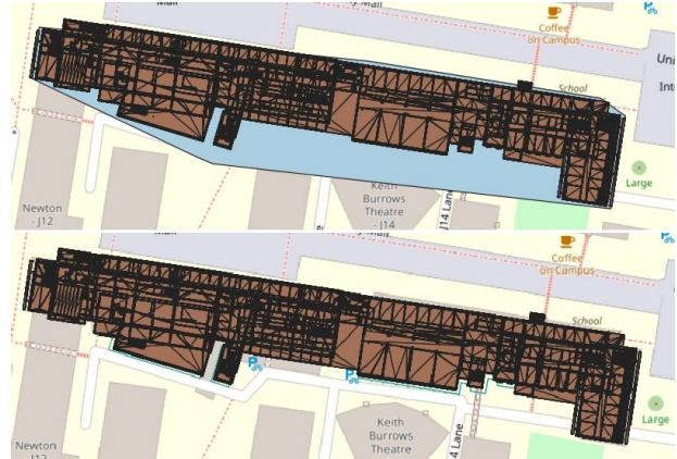
Figure 18 Georeferenced IFC model of the Red Centre. (Top) BIM model on top of the blue convex hull of the OSM feature used in the process. (Bottom) On top of the EM's footprint (green lines)
