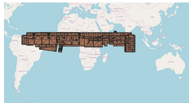
Figure 13 Result of the direct import of the raw BIM geometry in a GIS platform (QGIS)
