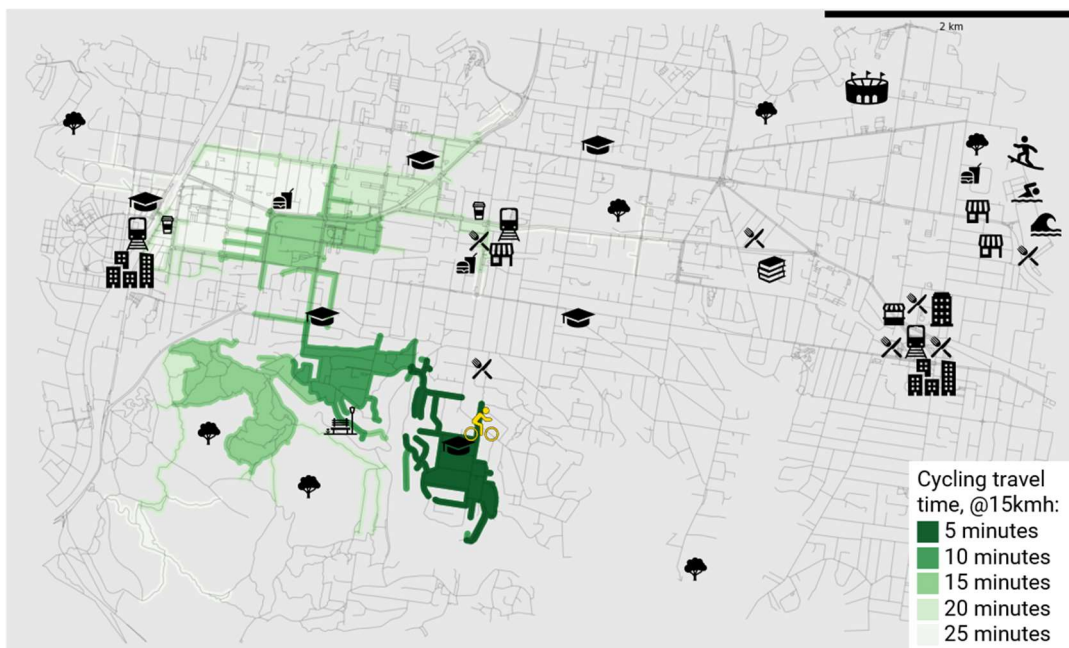
Figure 5: Isochrones of cycling access using the full road network (above) versus a low-stress network (below) showing the importance of considering cycling conditions
