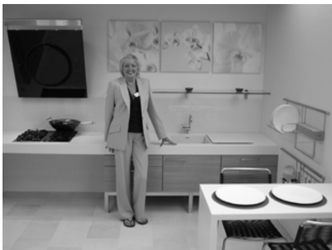
Figure 34: Lowered, wheelchair-accessible kitchen
