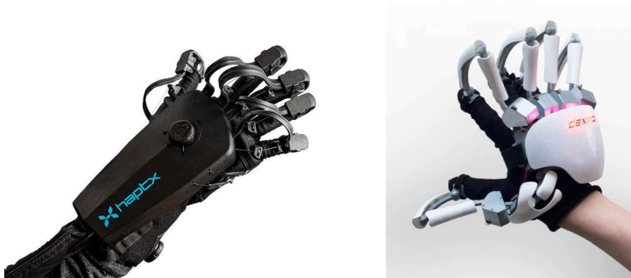
Figure 4: Haptic Feedback Gloves - Haptx DK2 [34] (left) and Dexmo [35] (right)
