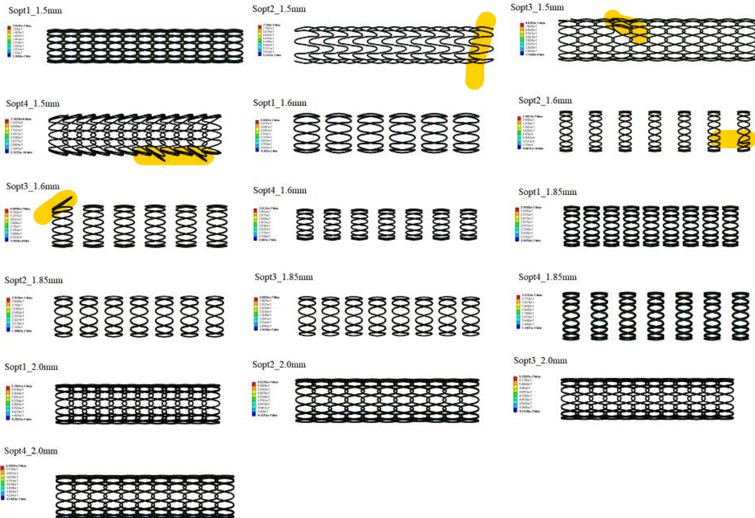
Figure 30 - Optimised stent deformation geometry and value
