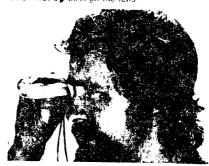
Use the left of the right eye as preferred. With both eyes open an optical liftusion makes the hairline appear to continue above the instrument frome, superimposed on the target. This improves reading accuracy and speed.
