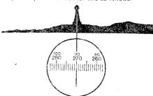
Take a reading with both eyes open and then close the free eye. If the reading does not change appreciably there is no disalignment of the eye axes, and both eyes can be kept open. Should there be a difference in the readings, keep the other eye closed and sight half-way above the instrument body. The hairline now rises above the instrument body and is seen against the target.
