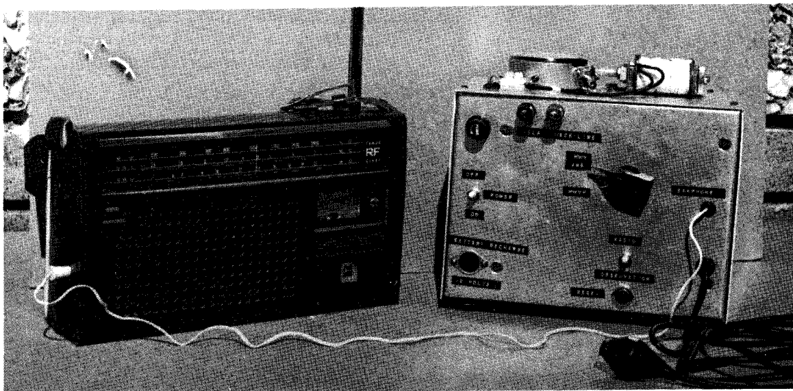
PLATE 8.1: TIME RECORDING APPARATUS SHOWING THE TRANSISTOR RADIO AND "TIMER."
