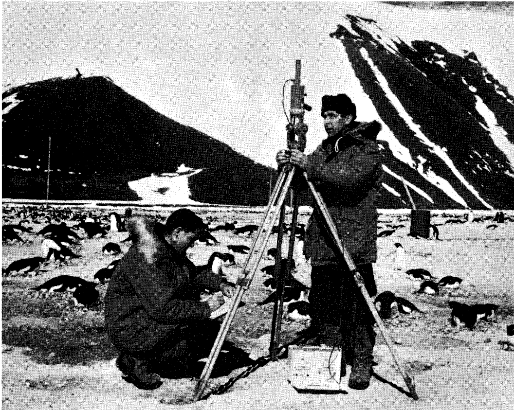
GYRO-THEODOLITE OBSERVATION AT HALLETT STATION, ANTARCTICA.
