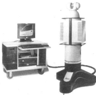
Figure 5.15: Leica Laser Radar System LR200 (after Leica 2002), similar to Metric Vision MV100B Coherent Laser Radar (CLR)
