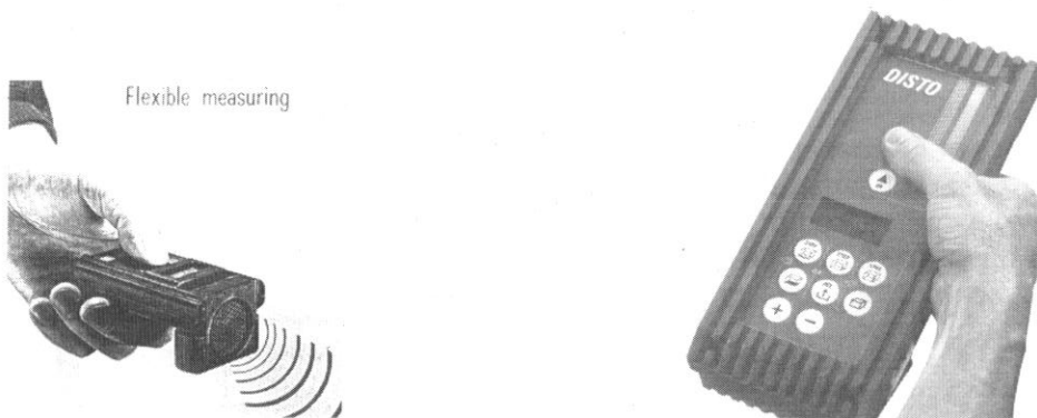
Figure 2.1: Accutape-S ultrasonic distance estimator (on left) and hand-held (electro-optical) laser meter DISTO by Leica (on right).
