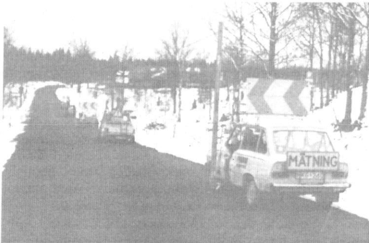
Figure 5.9: Motorised precise levelling in Sweden (after Becker 1979). In this case, two instrument vehicles and three staff vehicles can be seen.
