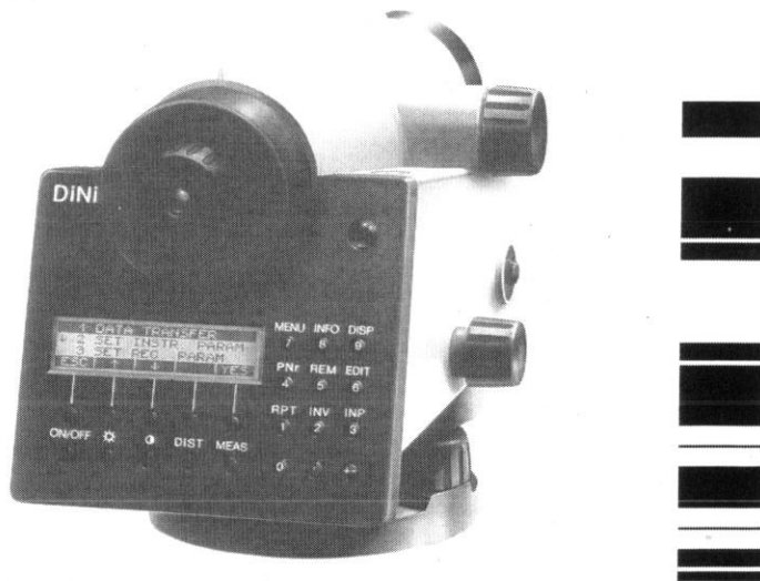
Figure 3.1: Zeiss (Trimble) DiNi10 digital levelling instrument (on left) and Zeiss bar code (on right)
