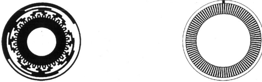
Figure 4.11: Basic layout of an absolute circle (on the left) and an incremental circle (on the right), after BEI (1987). The incremental circle also carries a reference mark (at the top). The innermost graduation of the absolute circle is equidistant, like the graduation of the incremental circle. Each graduation on the absolute circle can be identified by the unique binary code on the seven outer tracks.
