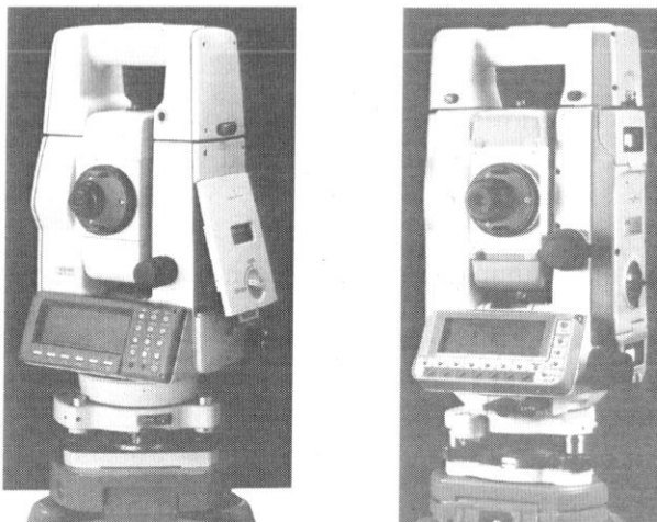
Figure 4.1: Two electronic tacheometers; Topcon GTS-701 on the left and Nikon DTM-720 on the right. Both instruments store data on PC-cards which slide into the side panels.
