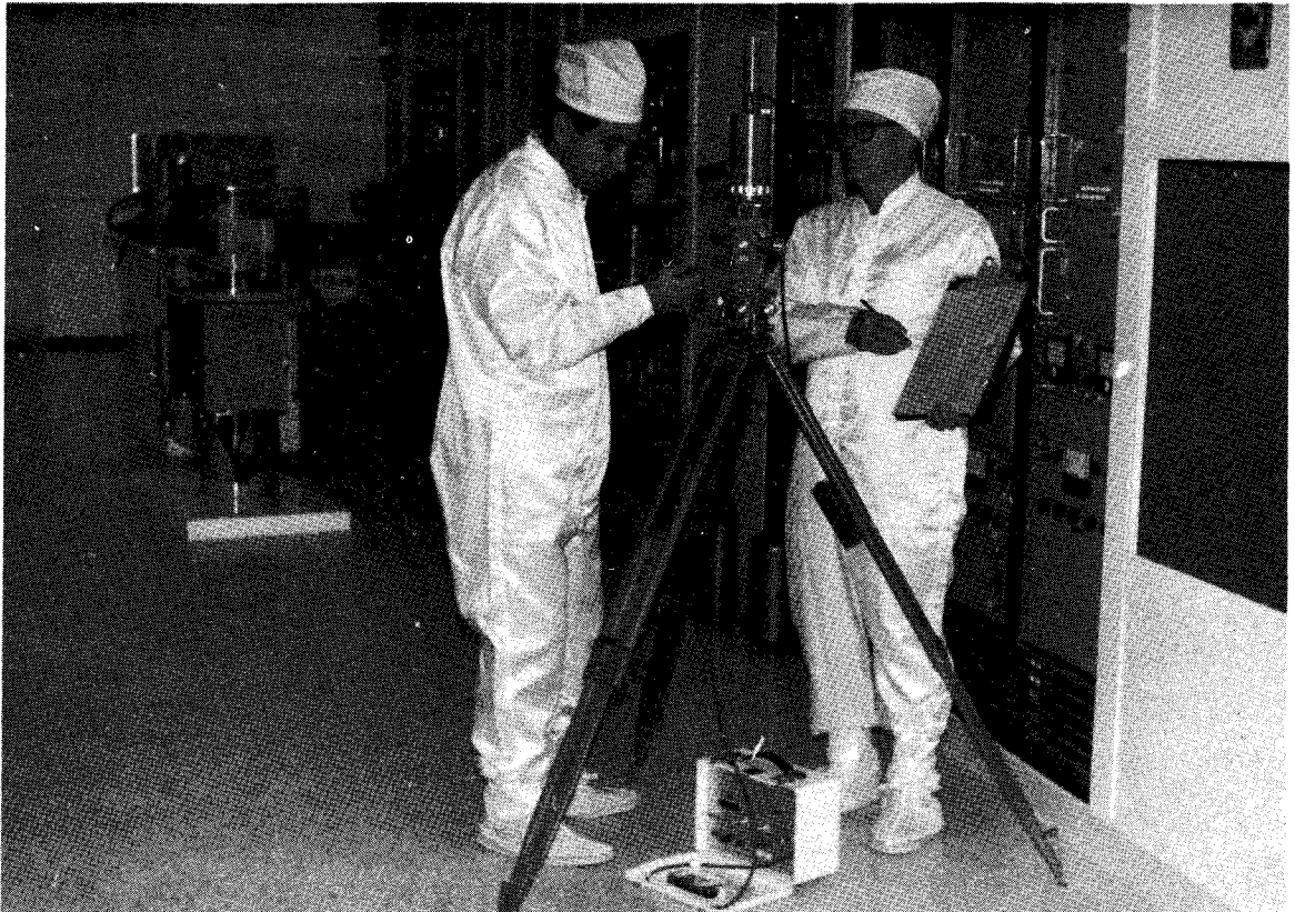
CALIBRATION OF AIRCRAFT GYROS BY GYRO-THEODOLITE IN THE "CLEAN ROOM" OF THE AVIONICS COMPLEX OF QANTAS AIRWAYS, SYDNEY.
