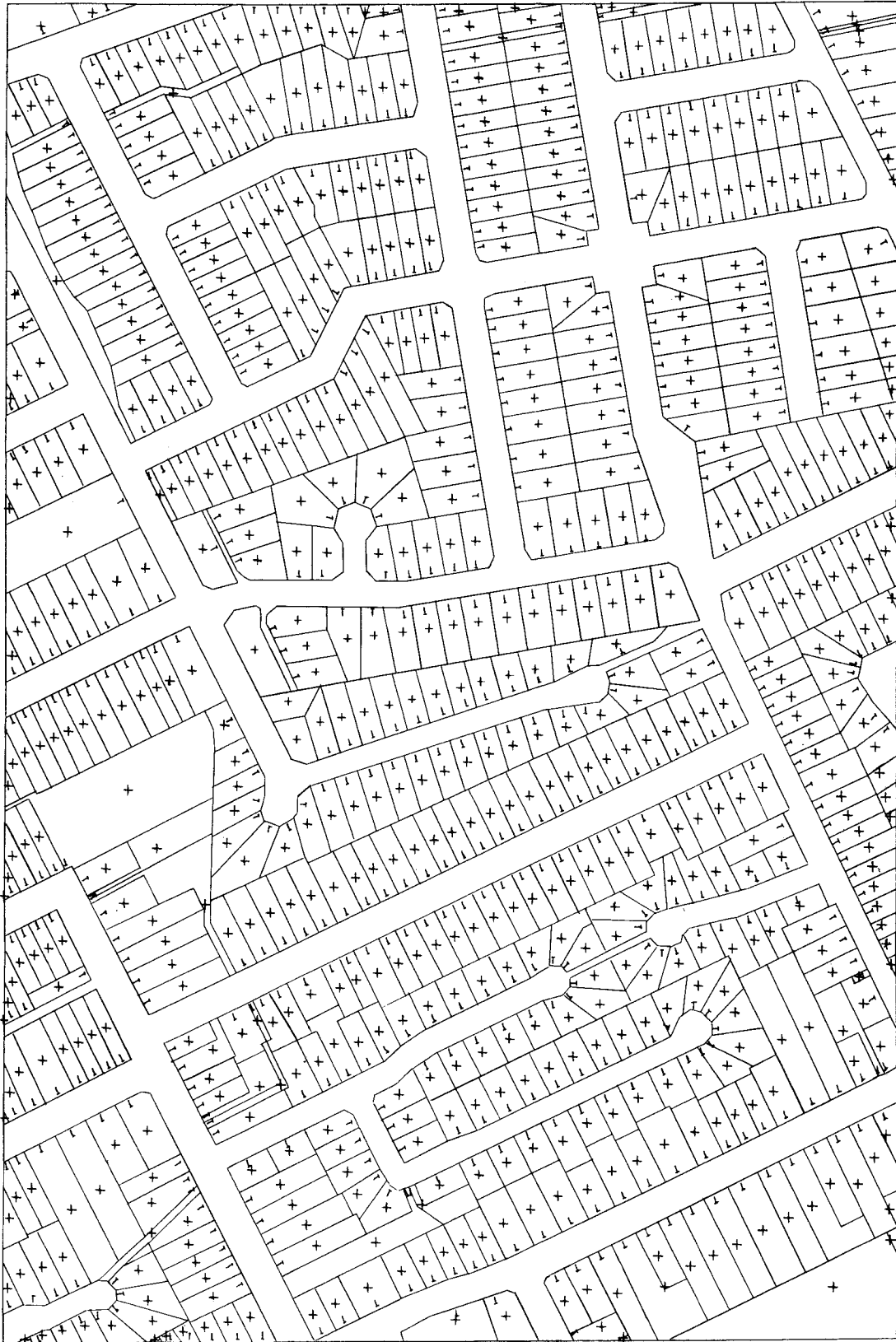
FIGURE C.2 Automatic placement of parcel identifier annotation computed from the parcel polygon file. Parcel centroid (+) parcel address point (I).
