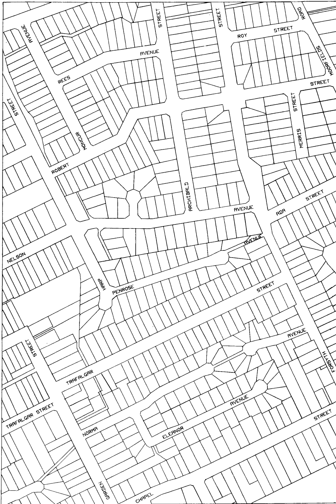
FIGURE C.4 Automatic placement of street name annotation computed from the digitized street segment network.
