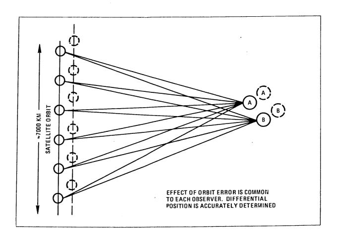
simultaneously tracked at all stations are used in the data reduction.
