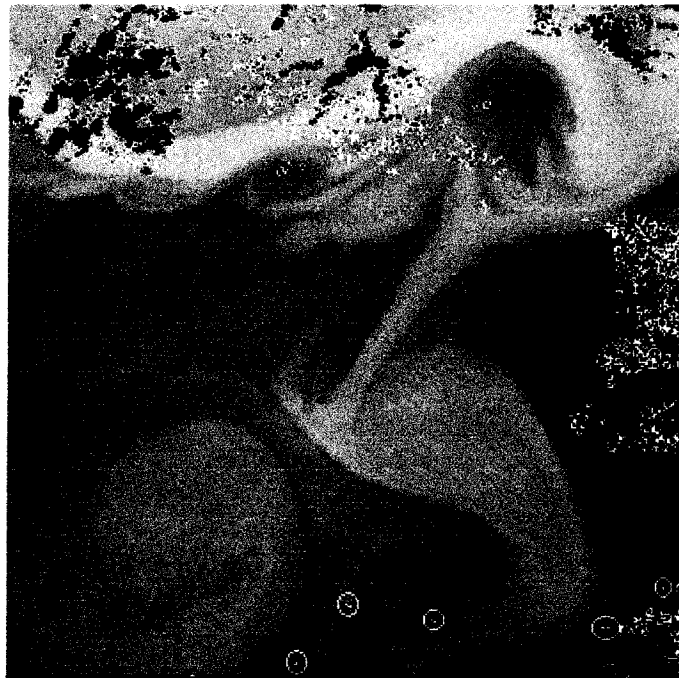
Figure 4.4 Image with the cloud mask computed with 5 \times 5 window, gradient strength threshold W_{thre} = 0.7W_{average} , and error ellipse roundness threshold Q_{thre} = 0.6 . The intensity criterion was not applied. The misinterpreted pixels are marked with white circles
