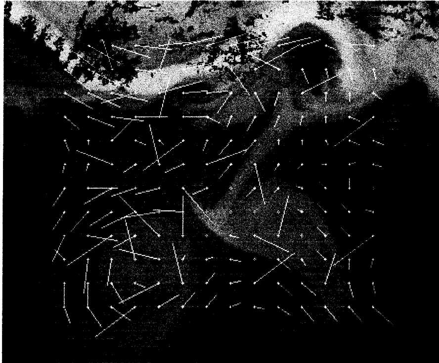
Figure 6.9 The candidate vectors of the maximum initial probability of each node of the testing candidate set containing randomly added erroneous candidates.
