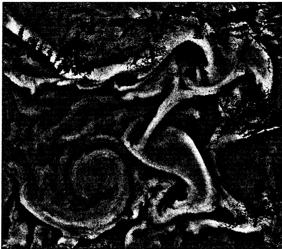
Figure 7.7 The image processed using a running average high-pass filter of 25 \times 25 pixels window. The original image is shown in Figure 5.1.
