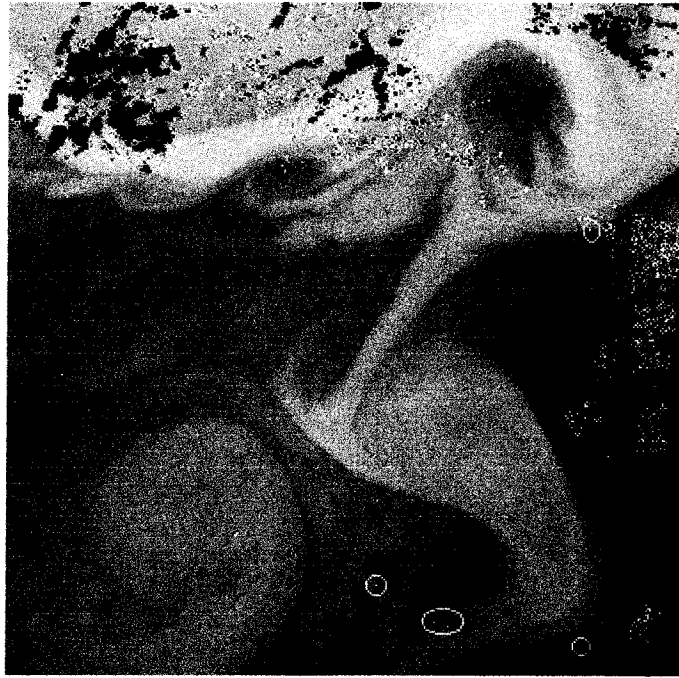
Figure 4.2.a Image with cloud mask computed with 3 \times 3 window, gradient strength threshold W_{thre} = 1.0W_{average} , and error ellipse roundness threshold Q_{thre} = 0.6 . The intensity criterion was applied. The misinterpreted pixels are marked with white circles
