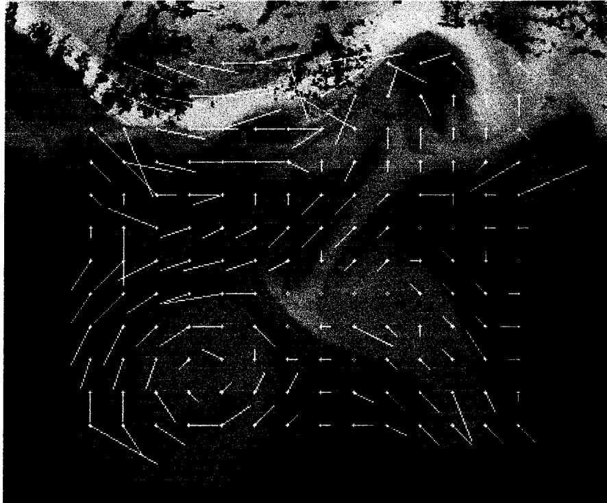
Figure 6.12 The candidate displacement vectors of maximum initial probability of each node selected based on the coarsely determined correlation matrices.
