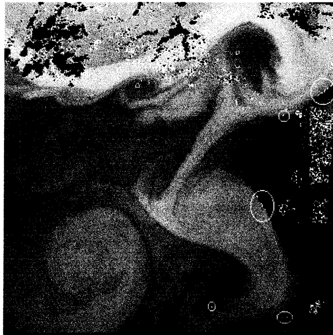
Figure 4.3 Image with the cloud mask computed with 5 \times 5 window, gradient strength threshold W_{thre} = 0.7W_{average} , and error ellipse roundness threshold Q_{thre}=0.1 . The intensity criterion was applied. The misinterpreted pixels are marked with white circles
