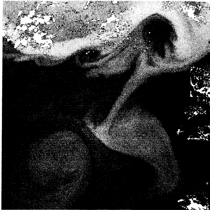
Figure 4.1. The image with a cloud mask determined with temperature thresholding. The detected cloud pixels are masked with white. The undetected broken clouds remain a dark grey colour.
