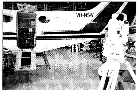
Figure 8.8 Determining the camera - antenna offset in the Hawker Pacific hangar.
