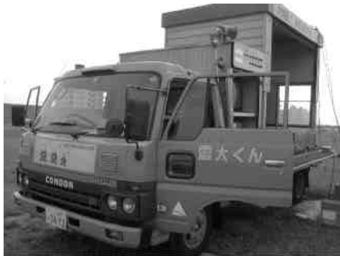
Figure 3.18 Earthquake shake-simulator truck used in the UNSW-MRI GPS Seismometer experiment.
