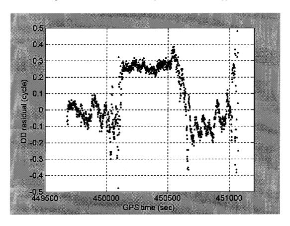
Figure 6-22. DD residuals of L1 carrier phase between receiver pairs R4 and R6
