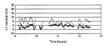
Figure 3-4a. L1 residuals for Glonass satellite pair PRN39-41 with (black) and without (grey) the Linear Combination Model
