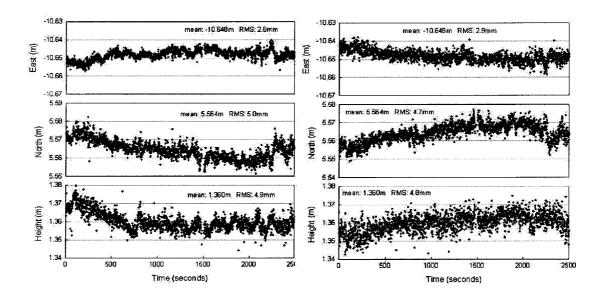
Figure 6-19. The East (upper plot), North (middle plot) and Height (lower plot) results for inverted carrier phase positioning (Left: type II, and Right: type I)
