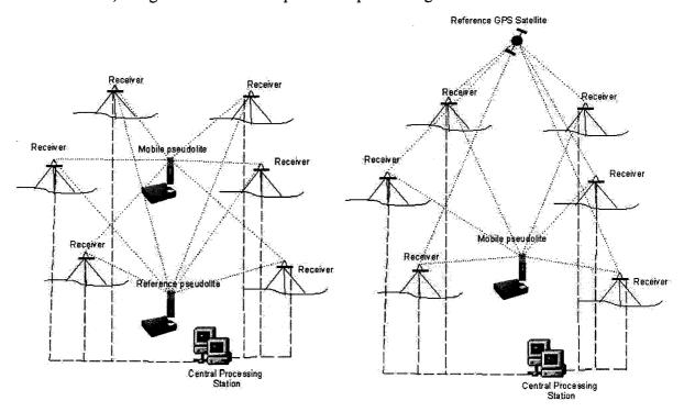
Figure 6-3. Inverted pseudolite positioning configurations (Left: two pseudolites, and Right: a pseudolite and a GPS satellite)
