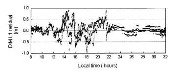
Figure 3-8c. Double-differenced L1 residuals for all the satellites pairs using the Distance-based Linear Interpolation Method
