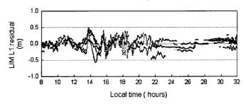
Figure 3-8d. Double-differenced L1 residuals for all the satellites pairs using the Linear Interpolation Method
