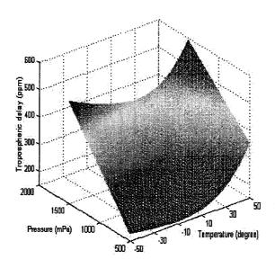
Figure 5-8. Pseudolite tropospheric delay with 50% RH
