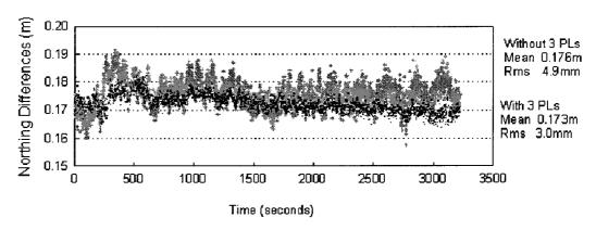
Figure 6-13. North component of the carrier phase solutions with GPS-pseudolite integration (black plot) and GPS-only (grey plot)
