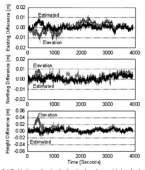
Figure 2-4. Positioning results using the elevation-dependent empirical stochastic model (grey) and the estimated stochastic model from residuals (black)
