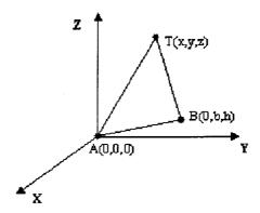
Figure 5-4. Set-up of the baseline (AB) and the transmitter (T)
