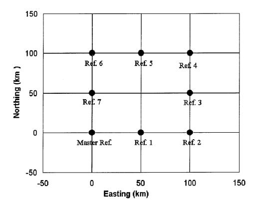
Figure 3-1. Configuration of the simulated reference station network
