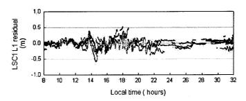
Figure 3-8f. Double-differenced L1 residuals for all the satellites pairs using the Least Squares Collocation Method proposed by Raquet (1998)
