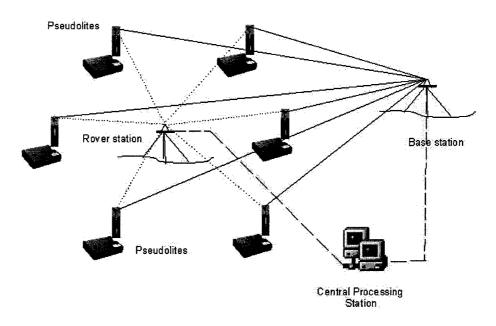
Figure 6-2. Configuration of a pseudolite-based positioning system
