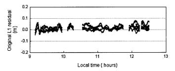
Figure 3-5b. Double-differenced L1 residuals for all the satellites pairs using the Linear Combination Model
