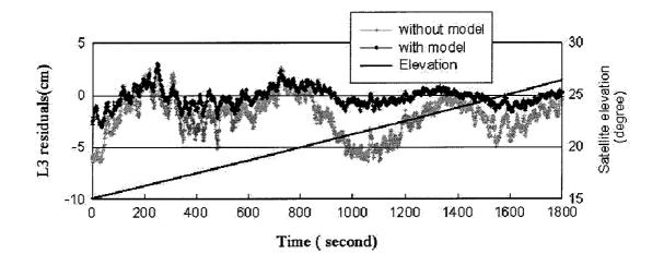
Figure 4-11. Residual tropospheric delay modelling for satellite pair 16-25
