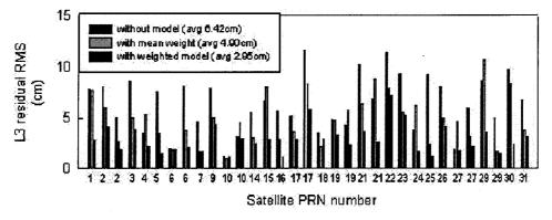
Figure 4-16. Improvement of L3 residual RMS, with and without bias modelling
