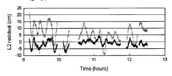
Figure 3-4b. L2 residuals for Glonass satellite pair PRN39-41 with (black) and without (grey) the Linear Combination Model
