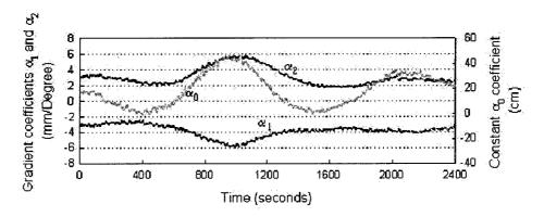
Figure 4-8. Constant and horizontal gradient coefficients for residual ionospheric modelling
