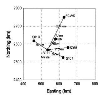
Figure 3-7. Configuration of the Taiwan multiple-reference station test network
