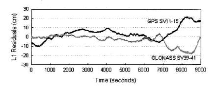
Figure 4-2. L1 residuals without model for GPS SV11-15, and Glonass SV39-41
