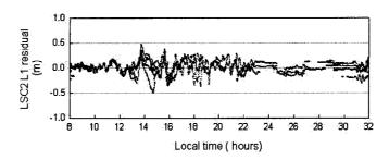
Figure 3-8g. Double-differenced L1 residuals for all the satellites pairs using the Least Squares Collocation Method proposed by Marel (1998)
