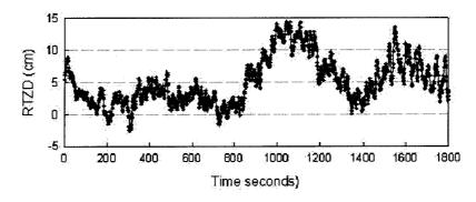
Figure 4-12. Estimated residual tropospheric zenith delay values
