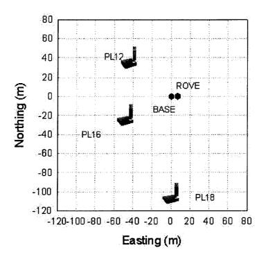
Figure 6-9. Location of instruments for the multiple pseudolite experiment
