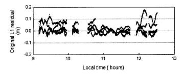
Figure 3-5c. Double-differenced L1 residuals for all the satellites pairs using the Distance-based Linear Interpolation Method
