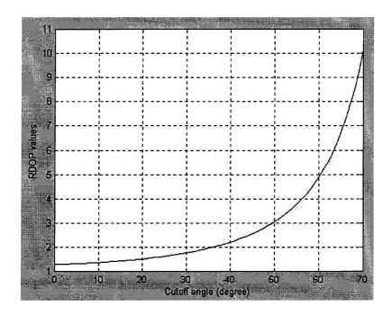
Figure 6-8. Minimum RDOP as a function of cut-off angle for four receivers
