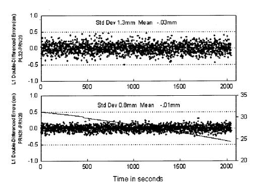
Figure 5-12 Noise level of the double-differenced carrier phase
