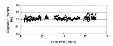
Figure 3-5d. Double-differenced L1 residuals for all the satellites pairs using the Least Squares Collocation Method
