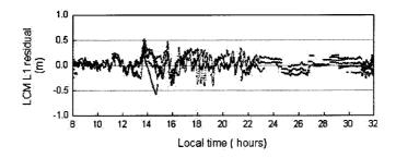
Figure 3-8b. Double-differenced L1 residuals for all the satellites pairs using the Linear Combination Model
