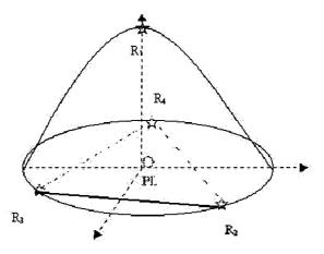
Figure 6-7. Optimum four-receiver array to minimise RDOP value
