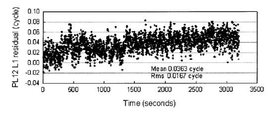
Figure 6-10. DD carrier phase residuals for PL12 – SV17
