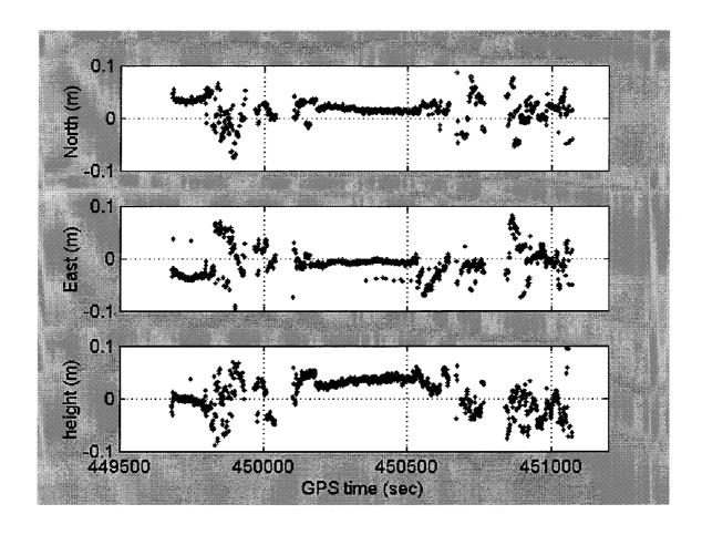
Figure 6-23. Kinematic positioning results in the inverted pseudolite test
