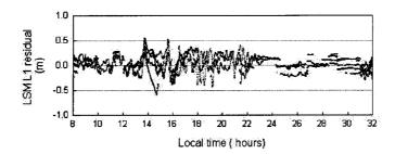
Figure 3-8e. Double-differenced L1 residuals for all the satellites pairs using the Loworder Surface Method (bivariate linear function fitting)
