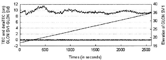
Figure 2-6.  $\nabla \Delta TEC$  and  $\delta TEC$  values for Glonass PRN 1 (Reference Glonass PRN 8, with highest elevation)
