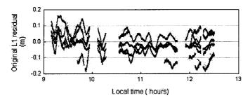
Figure 3-5a. Original double-differenced L1 residuals for all the satellites pairs
