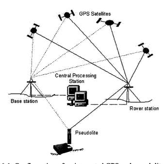
Figure 6-1. Configuration of an integrated GPS and pseudolite system
