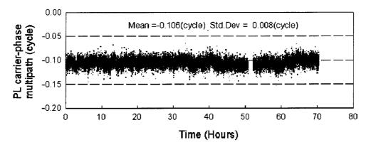
Figure 5-10. Multipath influence on the double-differenced carrier phase
