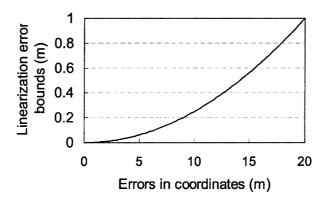
Figure 5-2. Linearisation error for the distance between pseudolites and user (200m)
