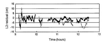
Figure 3-4d. L2 residuals for GPS satellite pair PRN16-11 with (black) and without (grey) the Linear Combination Model
