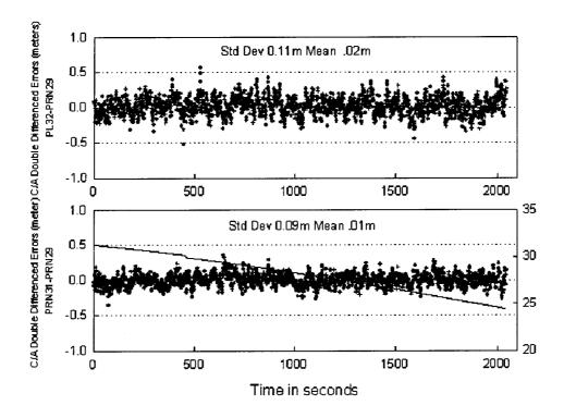
Figure 5-11 Noise level of the double-differenced pseudo-range
