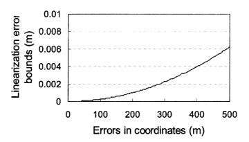
Figure 5-1. Linearisation error for the distance between satellites and user (about 20000km)
