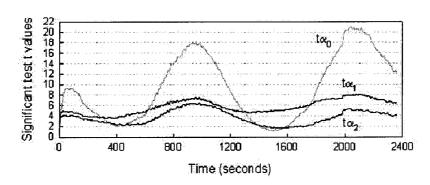
Figure 4-9. Significance test for residual ionospheric modelling parameters
