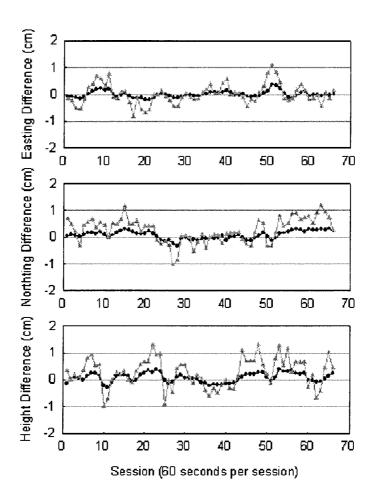
Figure 2-2. Rapid static positioning results for 1 minute sessions
