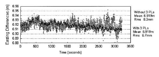
Figure 6-14. East component of the carrier phase solutions with GPS-pseudolite integration (black plot) and GPS-only (grey plot)
