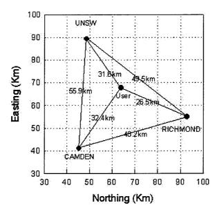
Figure 3-3. Configuration of the Sydney GPS/Glonass multiple-reference receiver network
