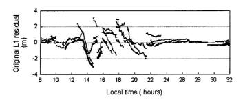
Figure 3-8a. Original double-differenced L1 residuals for all the satellites pairs
