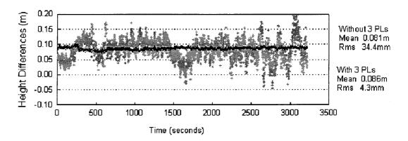
Figure 6-15. Height component of the carrier phase solutions with GPS-pseudolite integration (black plot) and GPS-only (grey plot)
