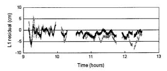
Figure 3-4c. L1 residuals for GPS satellite pair PRN16-11 with (black) and without (grey) the Linear Combination Model
