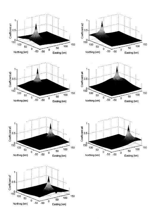
Figure 3-2b. Coefficients generated by the Distance-based linear Interpolation Method
