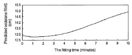
Figure 4-10. Optimal number of epochs for the residual ionospheric model (1 second sampling)
