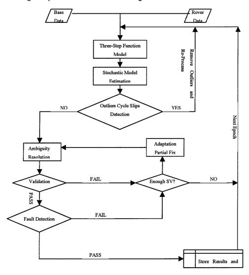
Figure 2-1 Float chart for the integrated procedure
