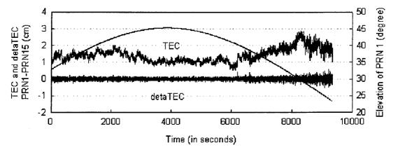
Figure 2-5.  $\nabla \Delta TEC$  and  $\delta TEC$  values for GPS PRN 1 (Reference GPS PRN 15, with highest elevation)
