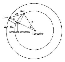
Figure 5-3 Example of pseudolite non-linear correction
