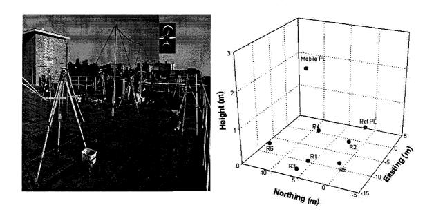
Figure 6-16. Location of instruments for inverted pseudolite positioning experiment
