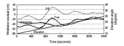
Figure 4-7. Residual ionospheric delay modelling for satellite pair 19-25
