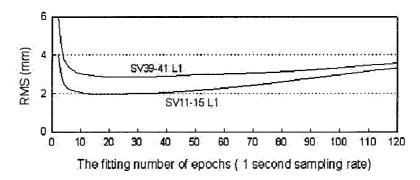
Figure 4-5. Optimal number of epochs for linear fitting for temporally correlated bias model
