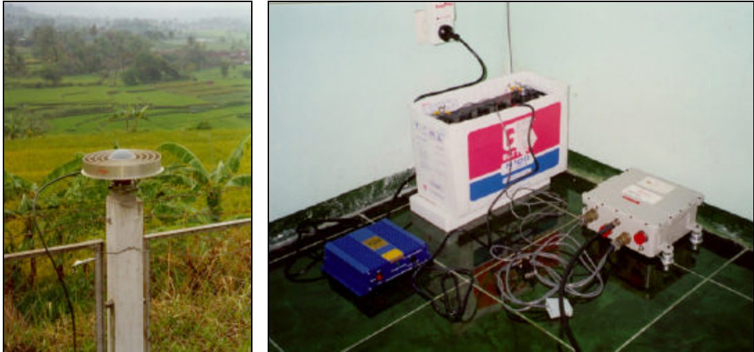
Fig. 2.17: Fiducial network: GPS antenna at Guntur (left) and GPS station equipment consisting of power surge protector, battery charger, battery and Leica CRS1000 GPS receiver (right)
