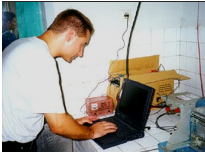
Fig. 2.15: The author at the Galunggung site: GPS equipment comprising battery charger, battery and Leica CRS1000 GPS receiver
