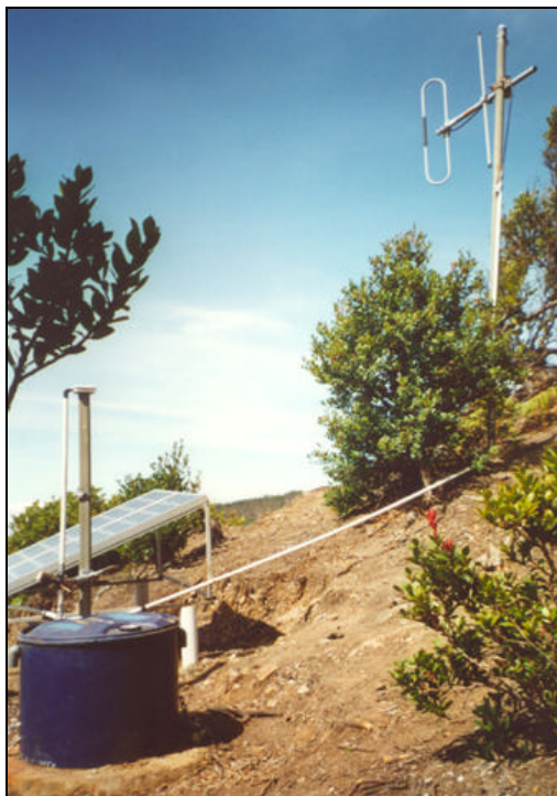
Fig. 2.11: Slave station setup on Gunung Papandayan (Nangklak): Solar panels, GPS antenna, plastic drum and radio antenna (left); battery, solar regulator, radio modem and GPS/PC module (right)
