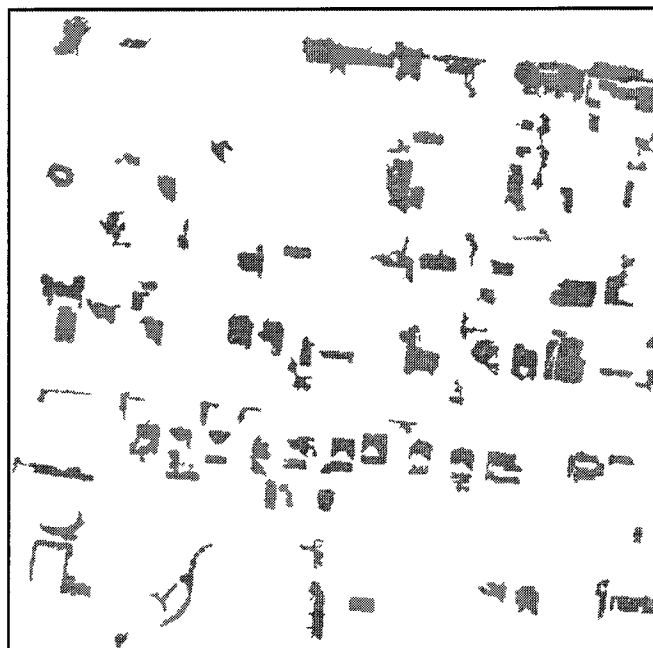
Figure 6.11 The pixels assigned as building class based on classification and DSM fusion
