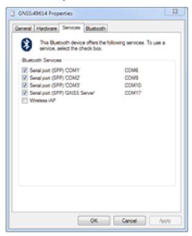
Applications that run on Windows devices (for example, the Trimble TerraFlex software) will see, in this example, COM6, COM9, COM10 and COM17. COM17 is the *GNSS Server* SPP port; it should NOT be selected for use by applications as it is used to supply positions to *Location Services* on the device. The *GNSS Server* port will reset to a default configuration each time it is connected, irrespective of any changes you make.
