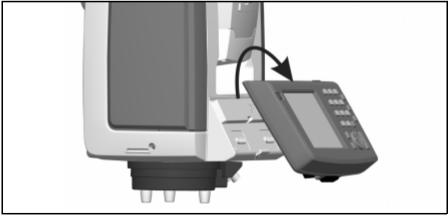
Figure 4.41 Detaching the Trimble CU
