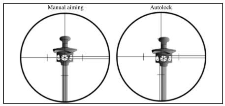
Figure 8.72 Difference between aiming manually and Autolock
