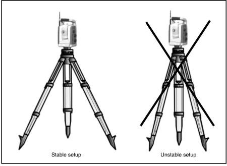
Figure 6.49 Tripod setup
