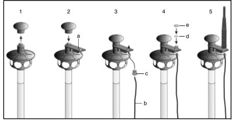
Figure 8.81 Fitting the antenna extension kit.
