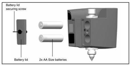
Figure 7.67 Target ID battery change
