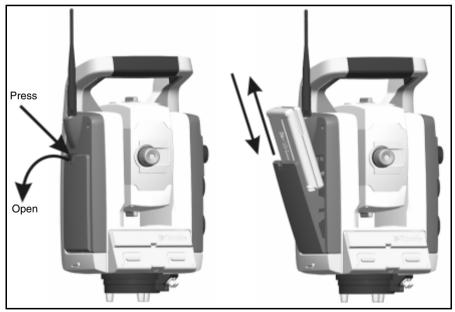
Figure 6.52 Removing and replacing the internal battery
