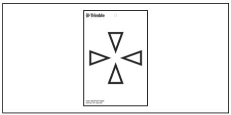
Figure 4.30 Adjustment target for DR 300+
