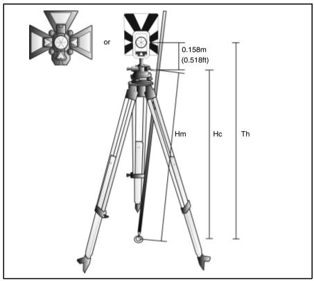
Figure 7.70 Target height measurement
