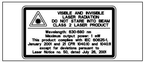
Figure 3.24 Laser pointer warning label
