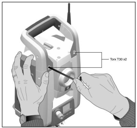
Figure 3.20 Removing the handle
