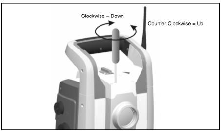
Figure 4.33 Vertical position adjustment
