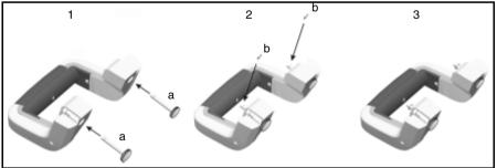
Figure 8.83 Fitting the new screws
