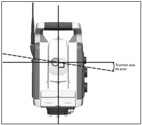
Figure 6.44 Trunnion axis tilt error
