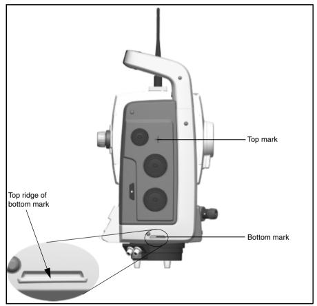
Figure 4.35 Instrument height marks
