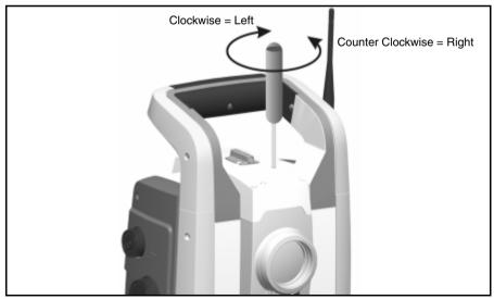
Figure 4.34 Horizontal position adjustment
