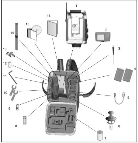
Figure 2.1 Position of items in the instrument case
