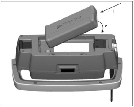
Figure 7.57 Attaching a battery to the Trimble Robotic Holder
