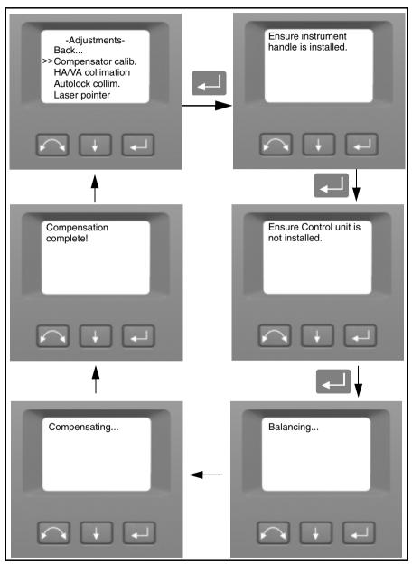
Figure 4.29 Compensator calibration routine
