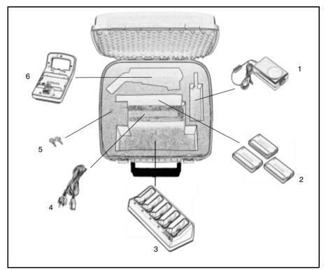
Figure 2.5 Contents of the battery kit accessory case
