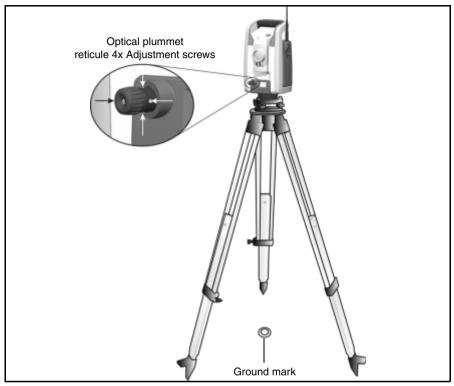
Figure 4.37 Optical plummet adjustment
