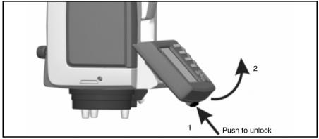
Figure 4.40 Detaching the Trimble CU
