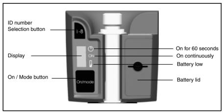
Figure 7.64 Target ID controls
