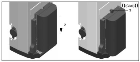
Figure 8.75 Fitting battery to external radio
