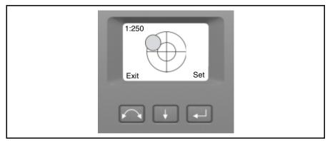
Figure 3.18 Electronic levelling screen in the face 2 display
