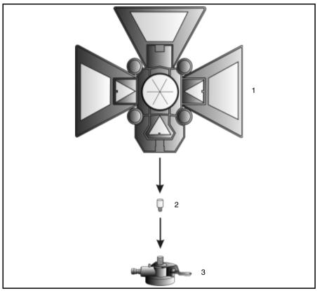
Figure 7.68 Assembling the traverse target
