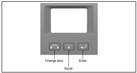
Figure 3.17 face 2 display and keyboard
