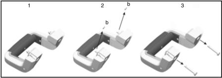
Figure 8.82 Removing the Torx screws
