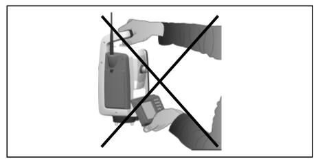
Figure 4.43 Wrong way to lift the instrument
