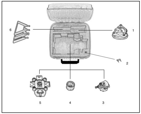
Figure 2.7 Contents of the traverse kit 1 accessory case
