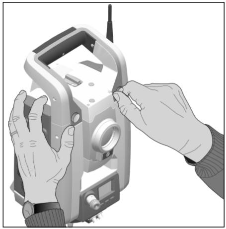
Figure 8.85 Securing the handle
