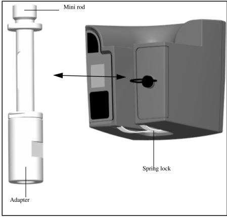
Figure 7.65 Fitting or removing the Target ID.
