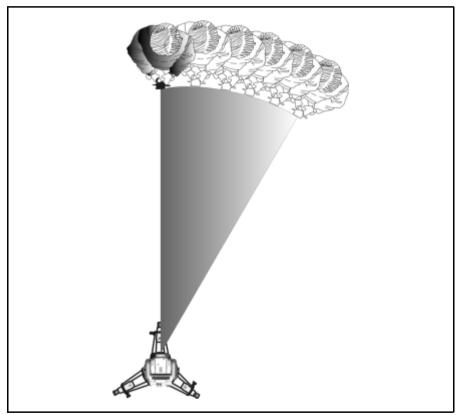
Figure 8.71 The Trimble S Series Total Station Autolock function.
