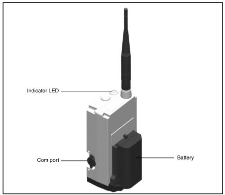
Figure 8.73 External radio 2.4 GHz
