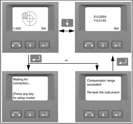
Figure 4.28 The levelling process
