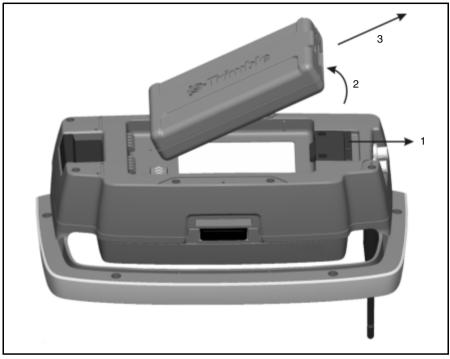
Figure 7.58 Detaching a battery from the Trimble Robotic Holder
