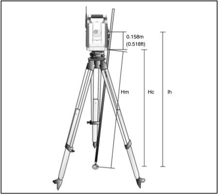
Figure 4.36 Instrument height measurement
