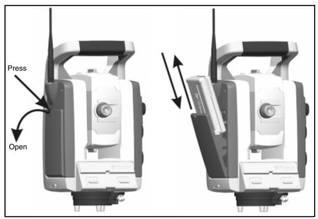
Figure 3.12 Removing and replacing the internal battery
