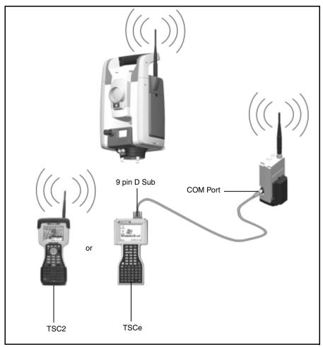
Figure 8.80 TSCe connected to the external radio for robotic measurements with the Trimble S Series Total Station.
