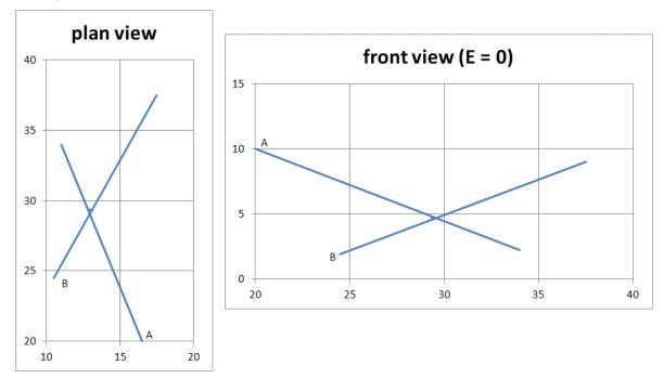
The distance between the two pipes is short so in both views above the shortest line appears to be very close to where the lines cross in each view. However if the distance was longer then the link line may not be so close to the crossing points. An exaggerated 3D view might then look like:
