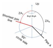
One angle in the spherical triangle is  $B_J$ - $B_A$ , the side opposite it is 90°, and the other two sides are  $ZA_A$  and  $ZA_J$ .
