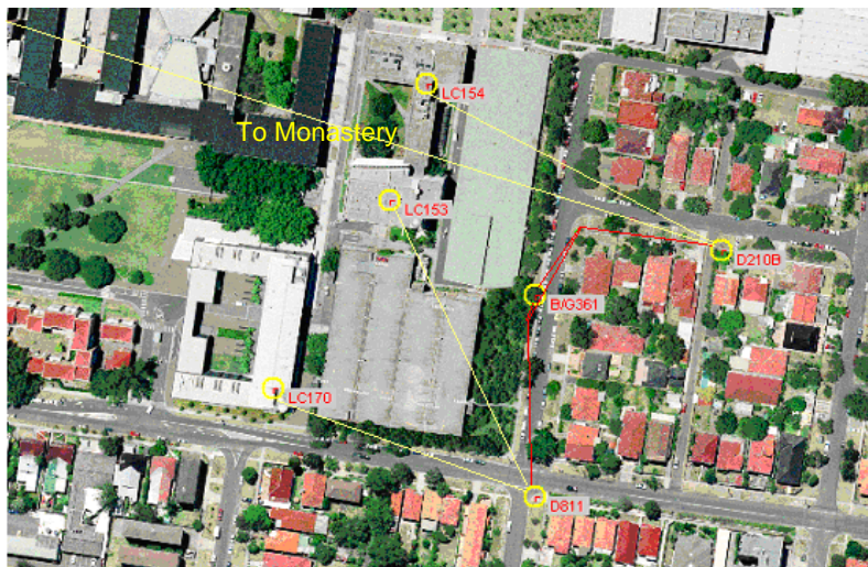
Fig. Plan of traverse. Traverse and radiations = Red Lines, Control target Sightings =Yellow lines.
