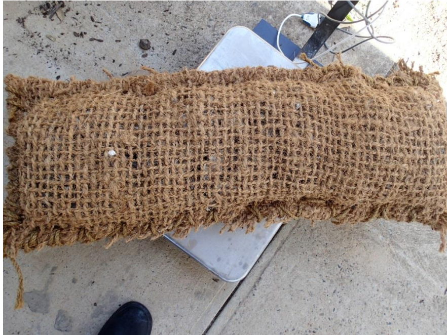
Figure 5-2: Example Single Oyster Shell Filled Bag
