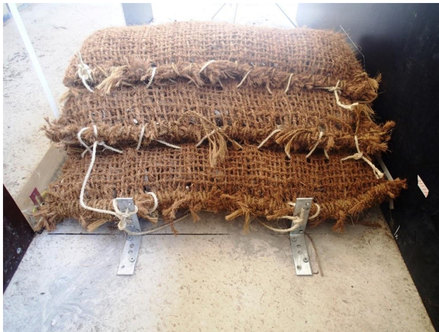
Figure 5-6: 3 Tier Oyster Shell Filled Bag Arrangement - Secured (Phase 2 Tests)
