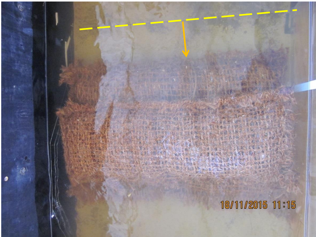
Figure 5-7: Before (Top) and After (Bottom) Photos Illustrating Displacement of Whole Structure (2 Tier High Structure) Note – Waves are Travelling from Top to Bottom
