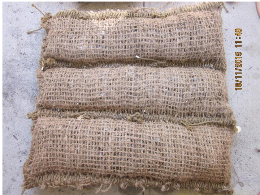
Figure 5-3: Example Triple Oyster Shell Filled Bag
