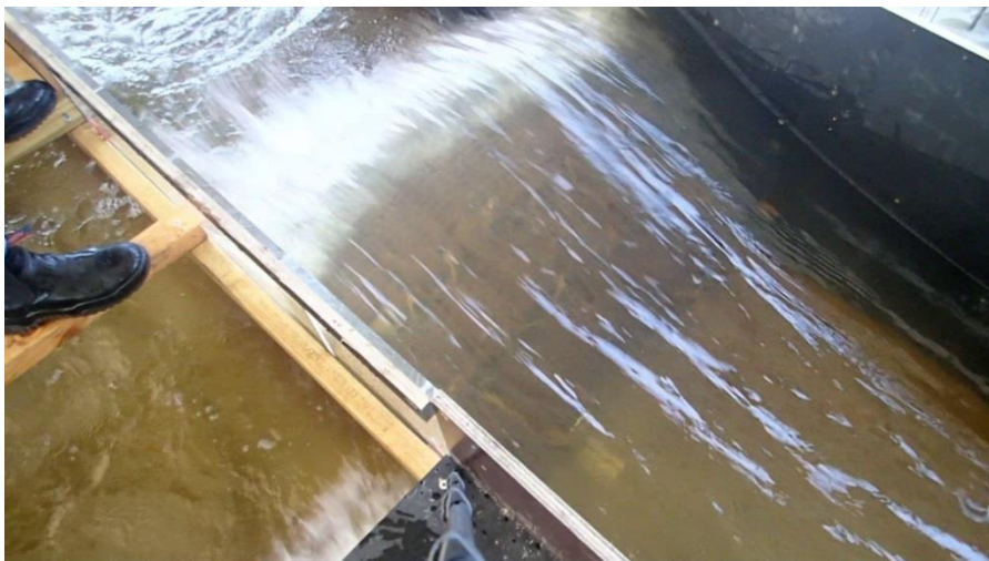
Figure 5-14: Example Photographs of Wave Attack on Oyster Shell Filled Bags During Phase 2 (Test 124) Note – Waves are Travelling from Right to Left
