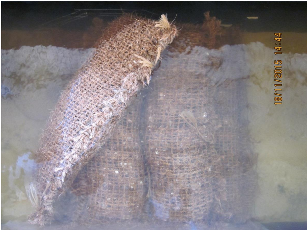
Figure 5-8: Before (Top) and After (Bottom) Photos Illustrating Complete Displacement of Crest Bag (3 Tier High Structure) Note – Waves are Travelling from Right to Left
