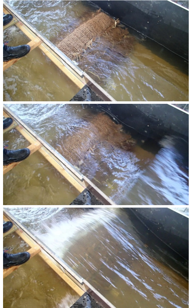
Figure 8 Wave attack on oyster shell filled bags during Phase 2 (3 tiers, WL = 0.40 m, T_p = 3 s, H_s = 0.28 m). Note – waves were travelling from right to left.
