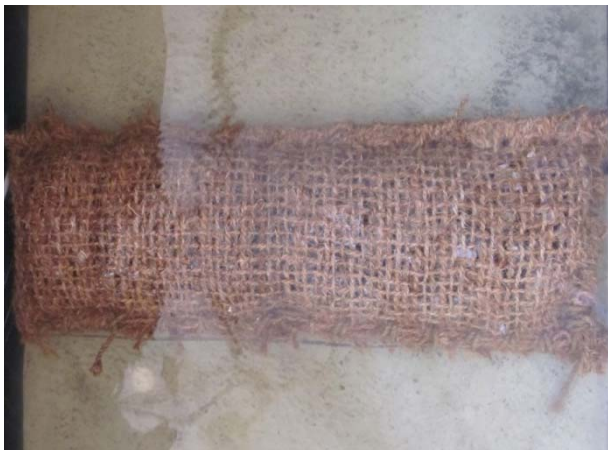
Figure 3 1 Tier oyster shell filled bag arrangement - unsecured (Phase 1 Tests)
