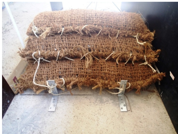
Figure 5 3 Tier oyster shell filled bag arrangement – secured (Phase 2 Tests)
