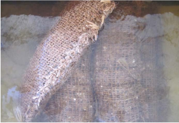
Figure 7 After complete displacement of crest bag (3 tiers, WL = 0.40 m, T = 2 s, H = 0.18 m). Note – waves were travelling from right to left.
