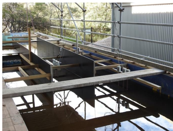
Figure 3 The experimental setup reveals the division of the 3 m wave flume into three small 1 m flumes, with wave probes in arrays of three used to separate incident and reflected wave heights.
