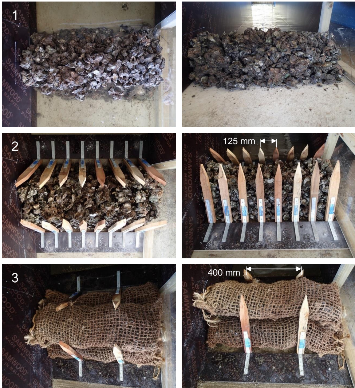
Figure 2.11 Different model configurations (top: Model 1, middle: Model 2, bottom: Model 3)
