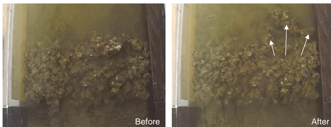
Figure 3.2 Failure of Model 1 with D=0.32 m, T=1 s, and H= 0.11 m
