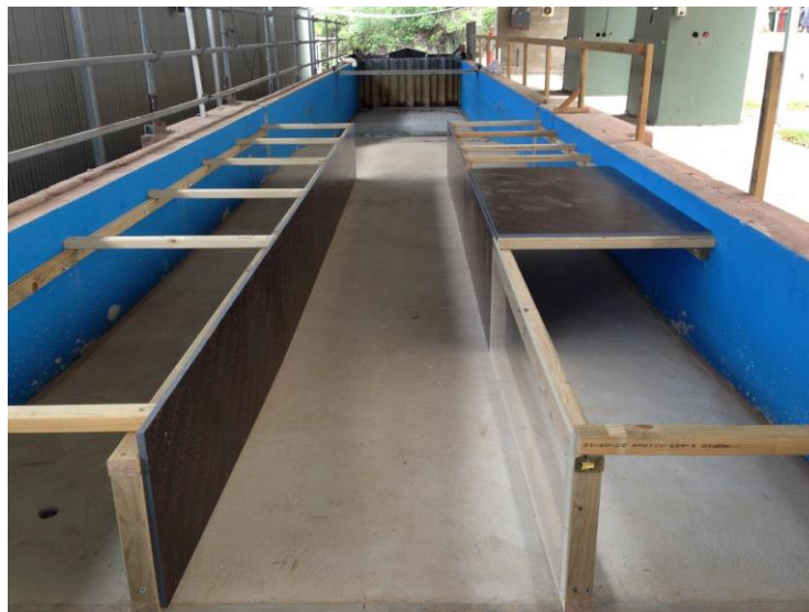
Figure 2.1 WRL 3 m wide wave flume, with 1 m wide mini-flume
