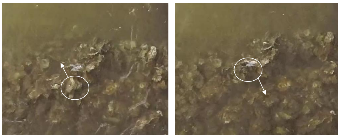
Figure 3.1 Rocking of clumps in Model 1 with D=0.32 m, T=2 s, and H= 0.08 m
