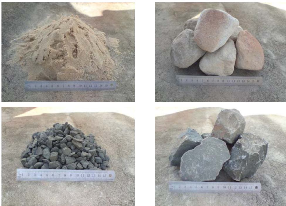
Figure 3. Test material used during this investigation. Upper left: sand; lower left: 10mm basalt; upper right: 80mm sandstone; lower right: 80mm basalt.
