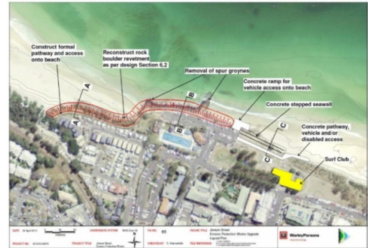
Figure 65 – Layout Plan – Rock Revetment and Stepped Concrete Seawall option
