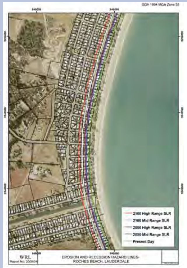
Figure 5.34 Erosion and recession hazard lines along the central section of Roches Beach. Source: Water Research Laboratory, UNSW
