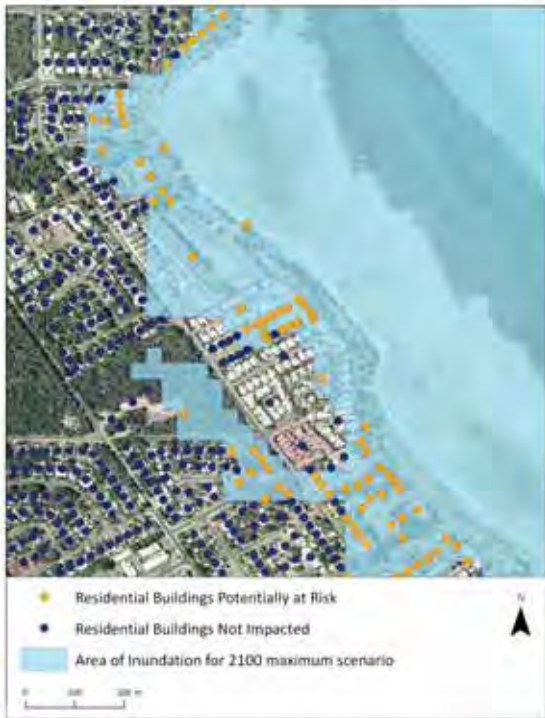
Figure 3.8 Example of overlay of NEXIS with an inundation footprint. Source: Geoscience Australia 2009
