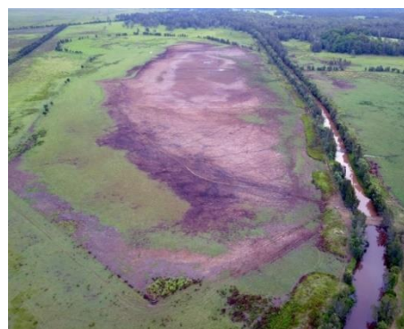
Figure 3 Yerbury's Scald in March 2018. A large acid scald with an elevation between -0.65 and -0.20 metres AHD located on the Clybucca floodplain. A large trunk drain (Seven Oaks Drain) runs along the northern side of the scald (to the right of the image). A low elevation weir can be seen across Seven Oaks Drain (bottom right of the image), constructed as part of remediation efforts in the 1990s.
