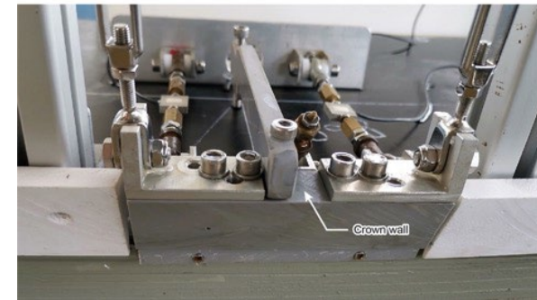
Figure 10 Crown wall section with load cells
