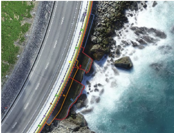
(a) Identification of the individual concrete block layers of the existing seawall
