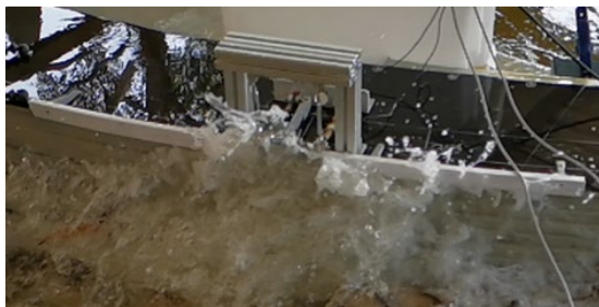
Figure 17 Wave hitting the crown wall during Test F1 (without concrete slab)
