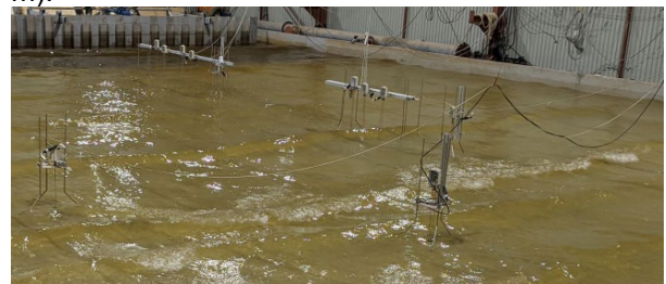
Figure 3: Physical model of wave transformation at WRL with the channel and not breakwaters.
