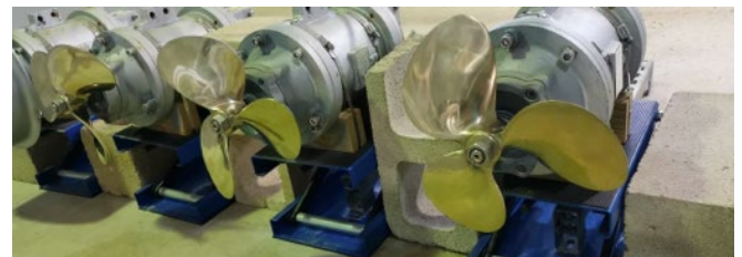
Figure 4 Four independently controlled propellers
