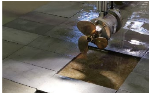
Figure 12 Concrete mattresses located directly under the propeller moved
