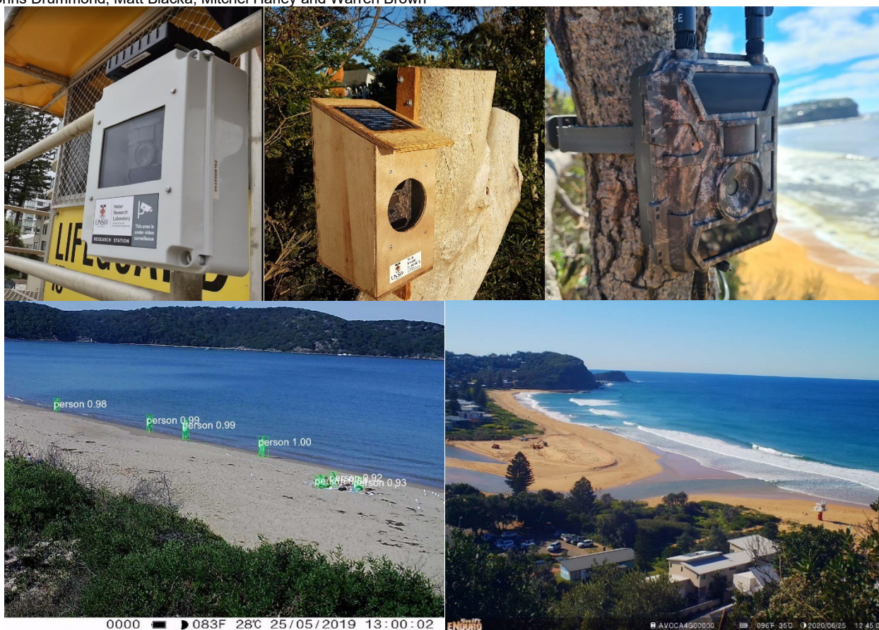
Figure 1 The WRL Beachstat smart camera system. Clockwise from top left: installation on a lifeguard tower; disguised inside a possum box to prevent vandalism; directly mounted to a tree; camera view of lagoon entrance at Avoca Beach, NSW; machine learning based user detection at Ettalong Beach, NSW.
