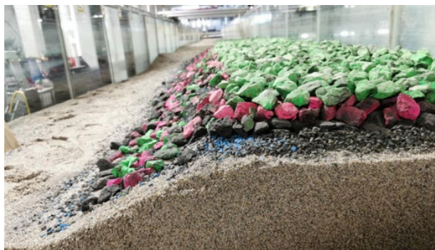
Figure 10: Example of Physical model test showing the performance of a falling rock apron using three layers of armour rock and an underlayer [7].
