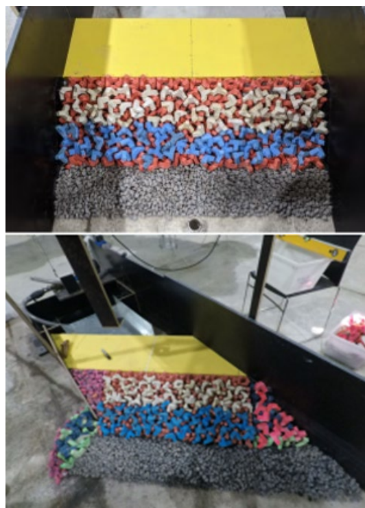
Figure 6: 2D Physical model tests were used to define site specific stability coefficients for waves approaching head on (top) and at 45^\circ (bottom).
