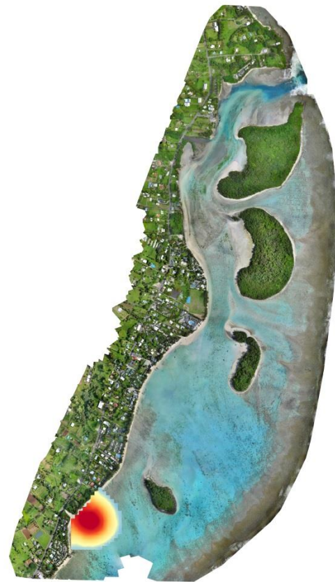
At end of 1 hour constituent release
