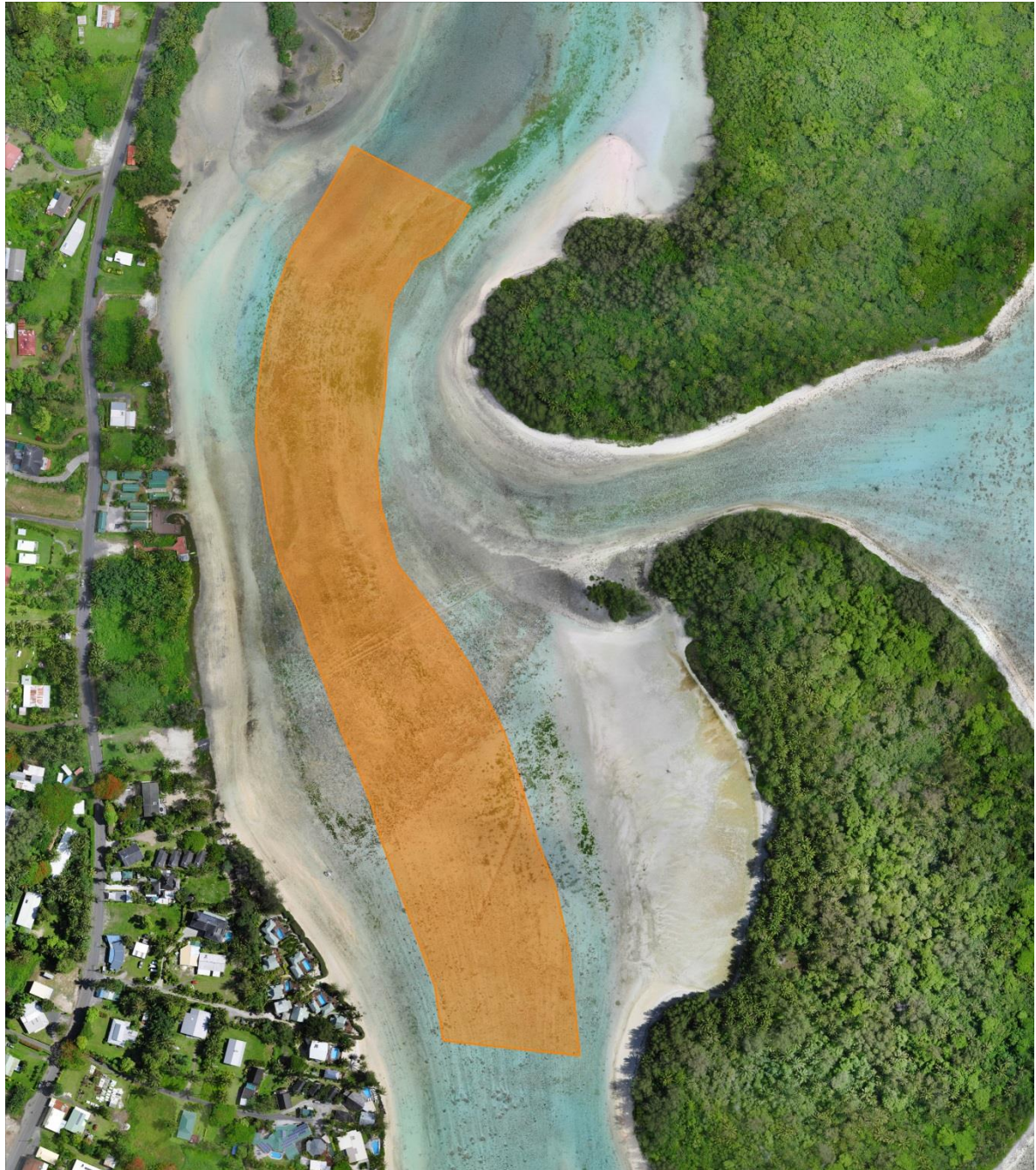
Figure 6.10: Area of bed lowered in model simulation
