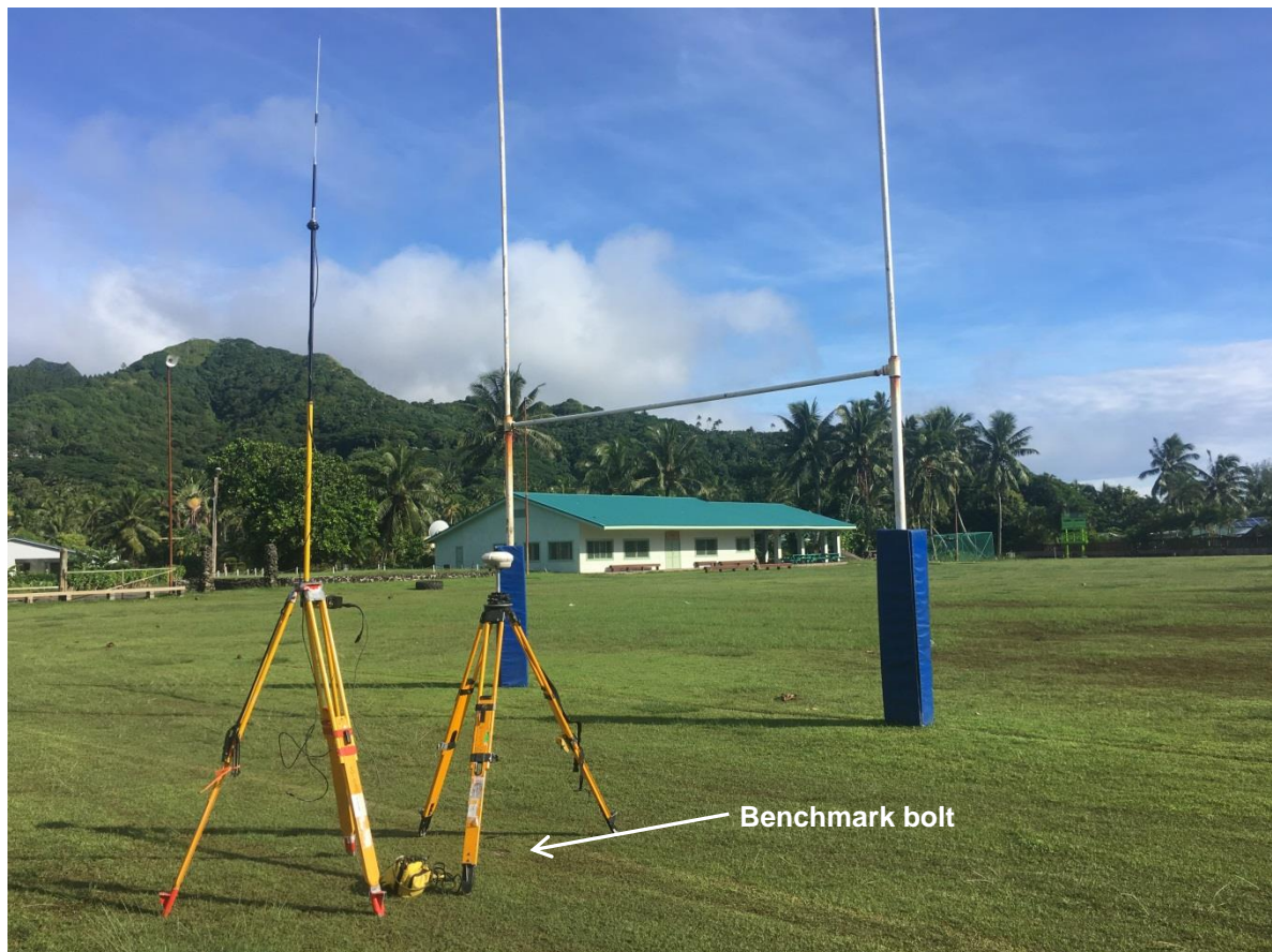
Figure 2.1: Location of Bolt 1 survey control bench mark, Nukupure Field
