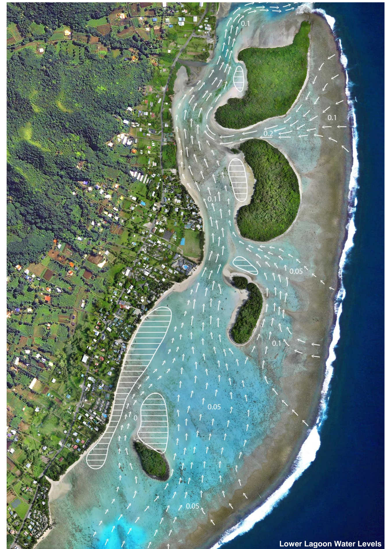
Figure 4.20: Indicative current patterns for lagoon hydrodynamic mode 2 (southwest to southeast wave directions)
