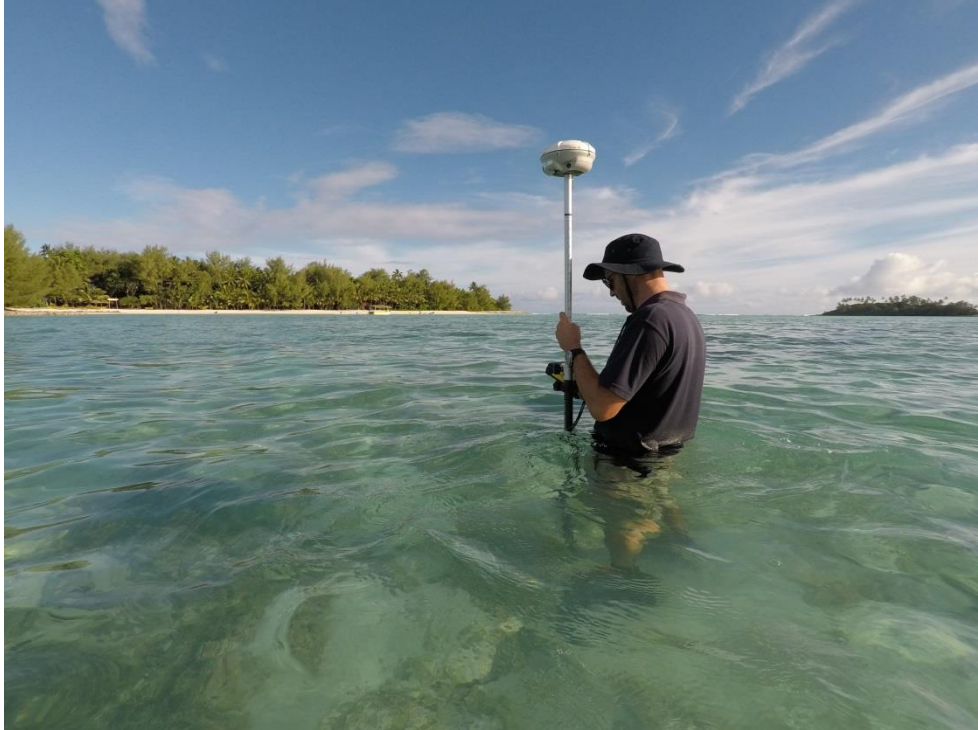
Figure 2.6: Wading RTK-GNSS bathymetric survey
