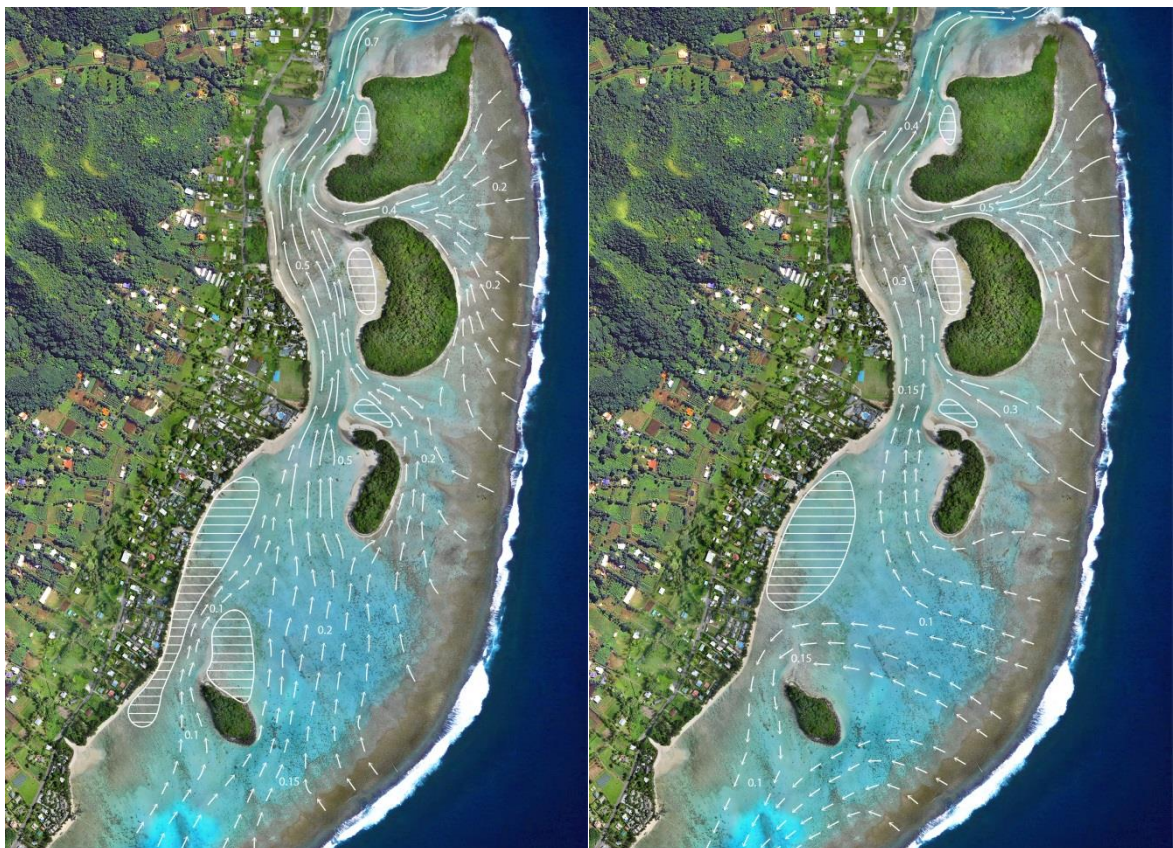
Figure 2: Different “Modes” of Lagoon flow patterns
