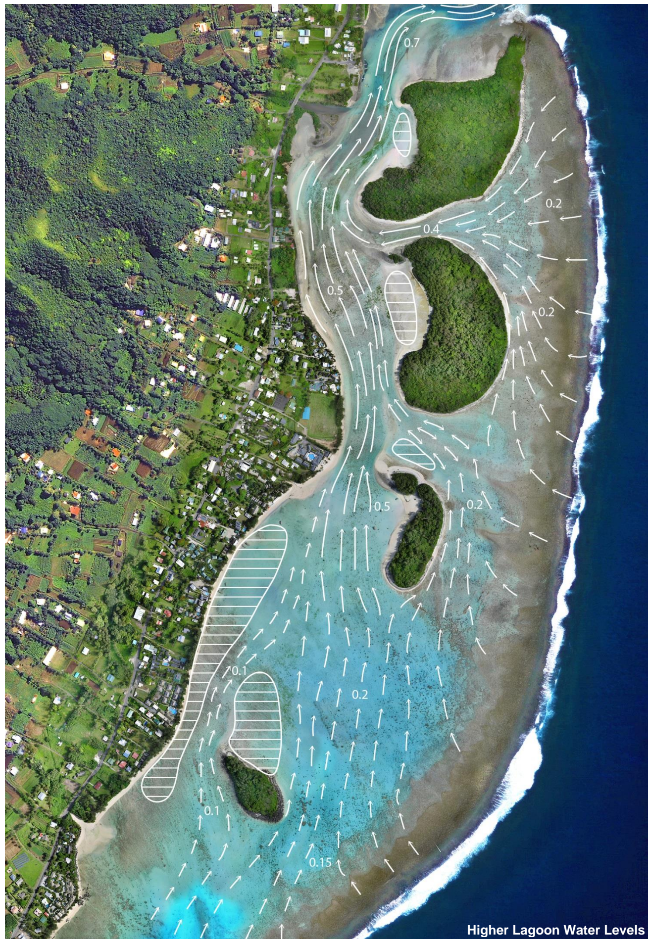
Figure 4.20: Indicative current patterns for lagoon hydrodynamic mode 2 (southwest to southeast wave directions)
