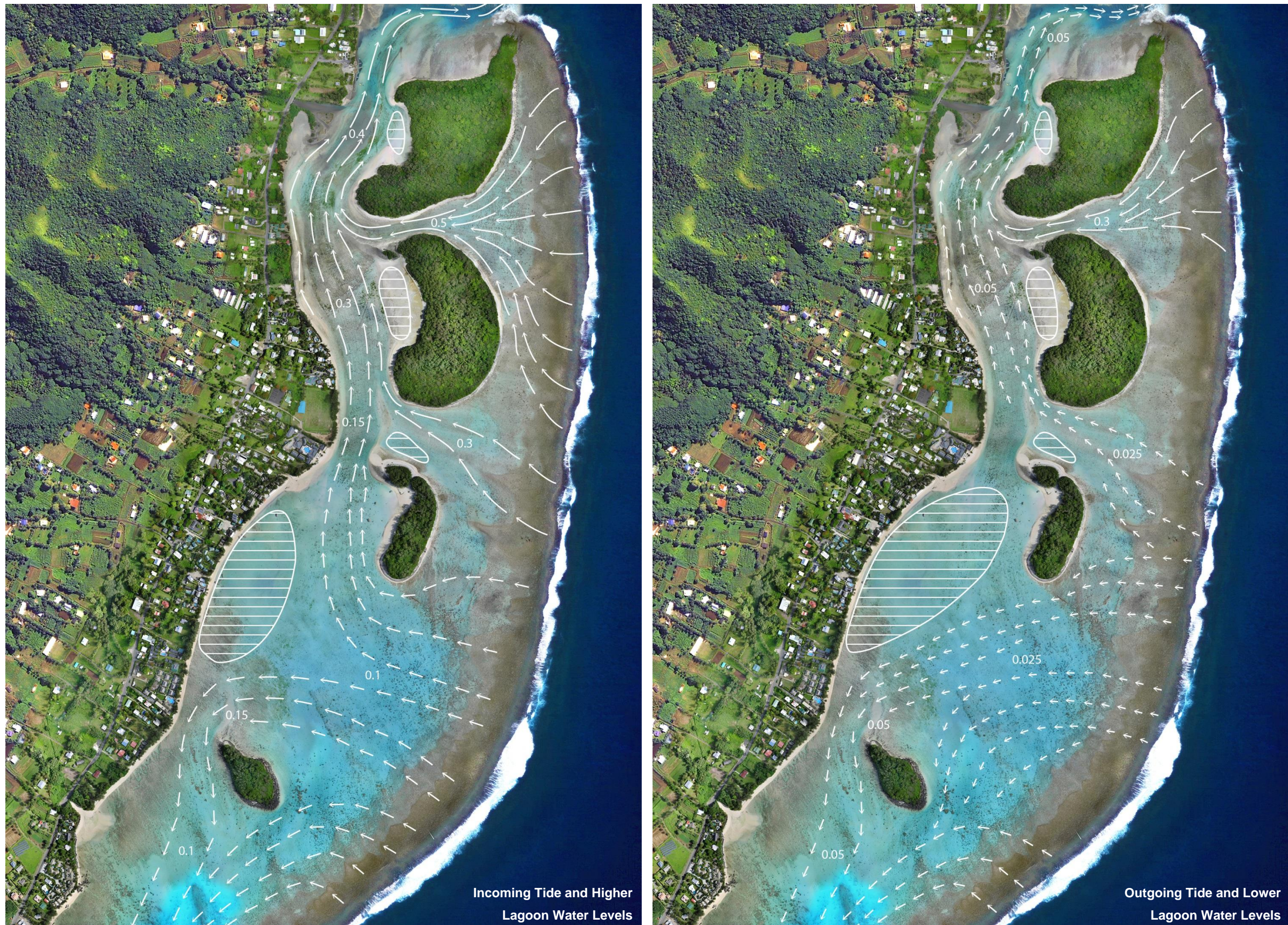
Figure 4.21: Indicative current patterns for lagoon hydrodynamic mode 2 (west through north to northeast wave directions)
