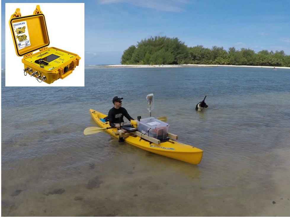
Figure 2.4: Bathymetric survey kayak with CeeScope single beam echosounder
