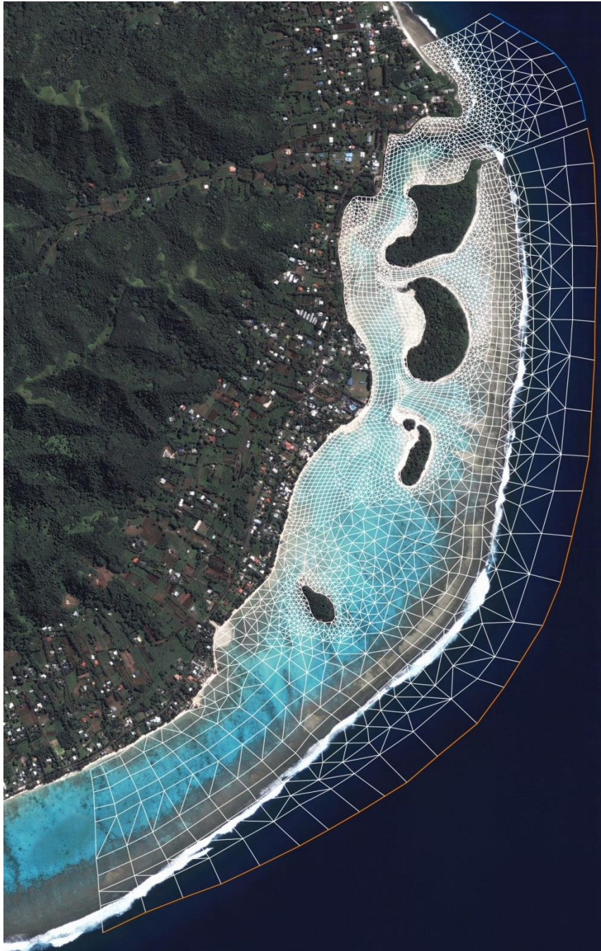
Figure 6.5: RMA-2 numerical model mesh
