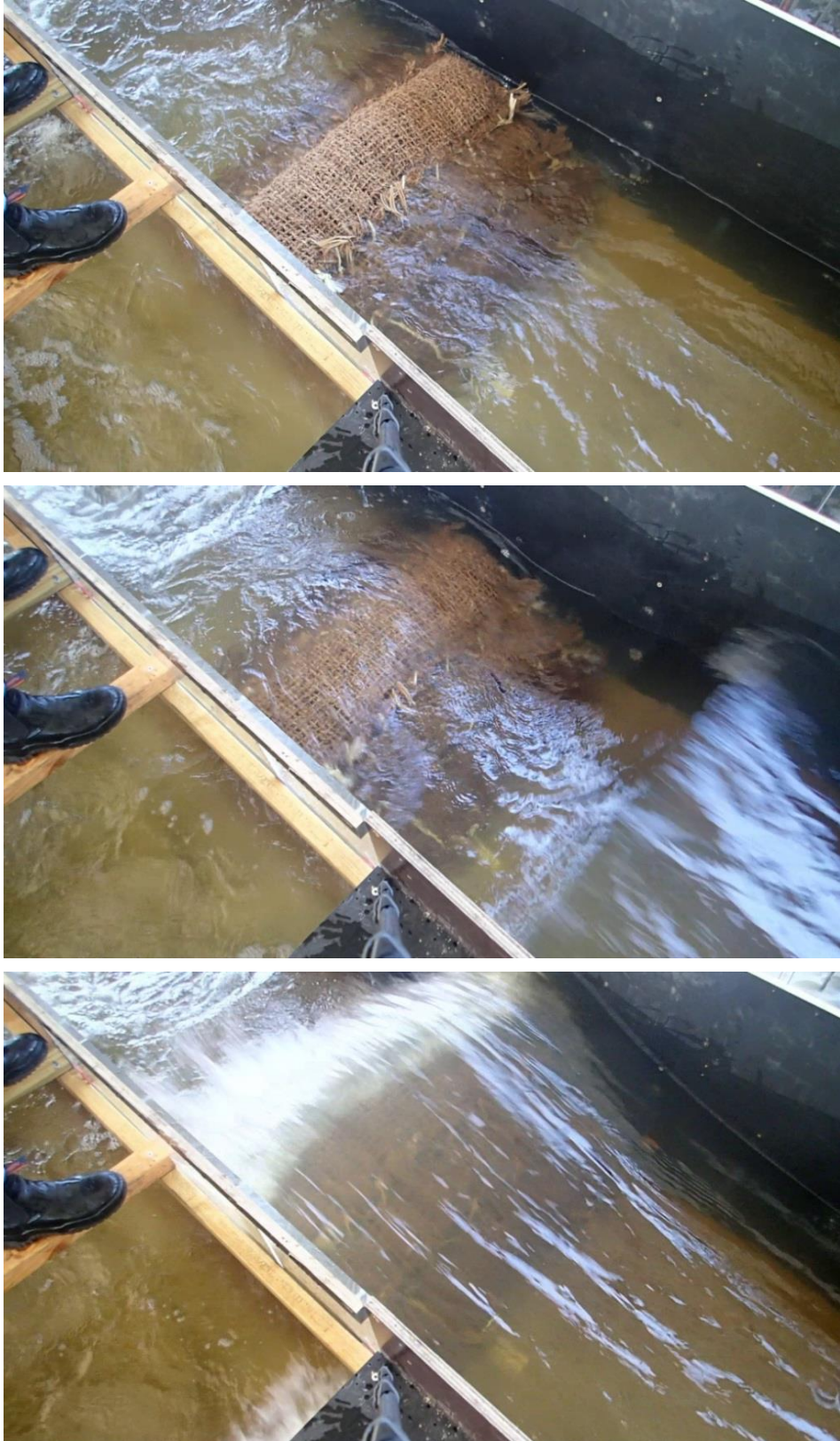
Figure 2.3 Example photographs of wave attack on oyster shell filled bags during Phase 2
