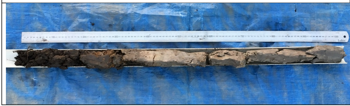
Figure C.25: Soil Profile During Field Survey
