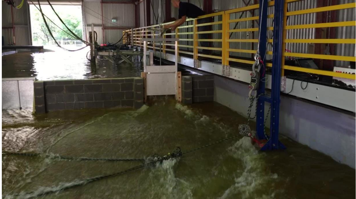
Figure 5-4: Rapid filling of WRL's test tank (wave basin). The winch assembly is also shown.
