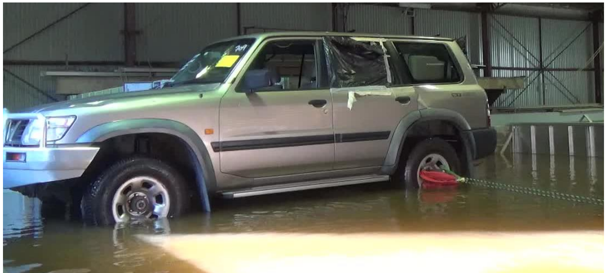
Figure 5-2: Nissan Patrol in WRL’s wave facility, preparing for a winch test from the rear axle
