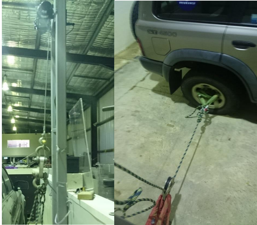
Figure 5-3: Winch assembly in WRL Lab#2, including (a) framework, winch and dynamometer, (b) pulley and wheel attachment
