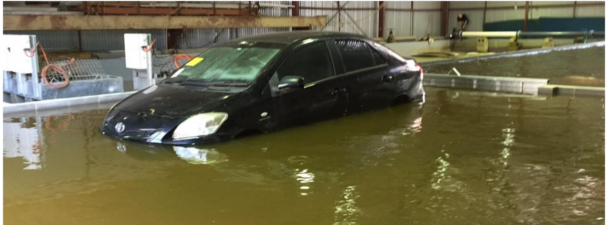
Figure 5-5: Toyota Yaris in WRL's wave basin facility, in 0.6 m water depth with rear wheels clear of the floor
