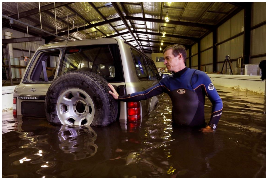
Figure 5-6 The lead author demonstrating zero traction at the rear wheels for the Nissan Patrol 4WD in WRL's Lab#2 testing tank. Water depth is approximately 1.0m.
