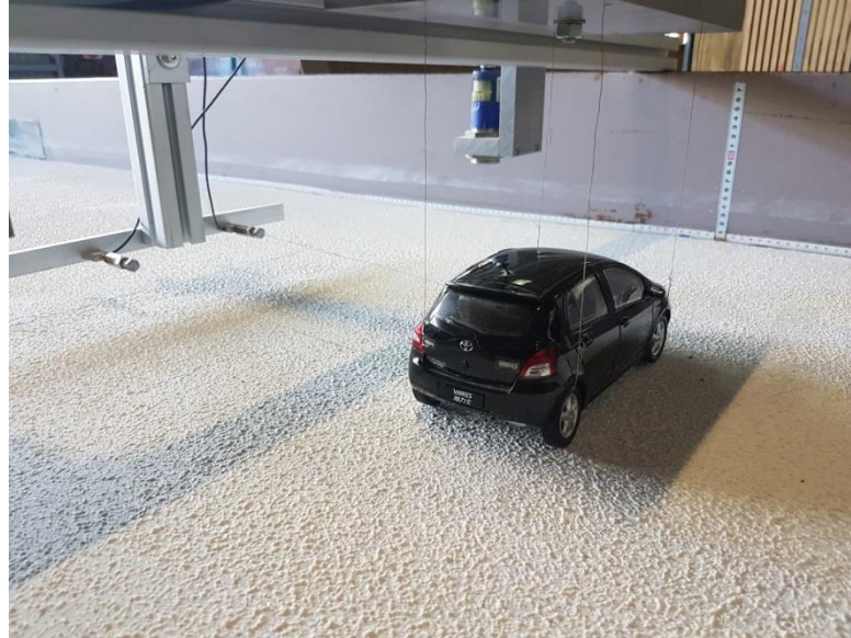
Figure 6-1: Test assembly for testing of the horizontal hydrodynamic forces. Flow is from the left of the picture
