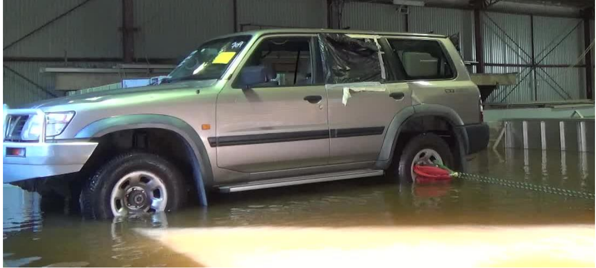
Figure 4-2: Nissan Patrol in WRL’s wave basin facility, preparing for a winch test from the rear axle
