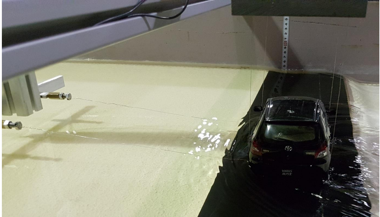
Figure 6-3 Testing of the model on a broad crested weir
