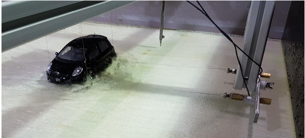
Figure 6-4: Testing of the model in supercritical flows d = 0.225\text{m} , v=4.0\text{m/s} (prototype), C_D = 1.86 , Fr = 2.66
