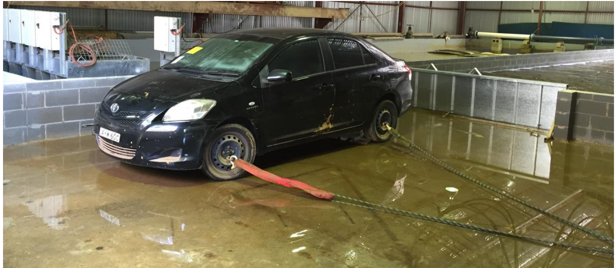
Figure 5-1: Toyota Yaris in WRL’s test facility, preparing for a winch test from both axles
