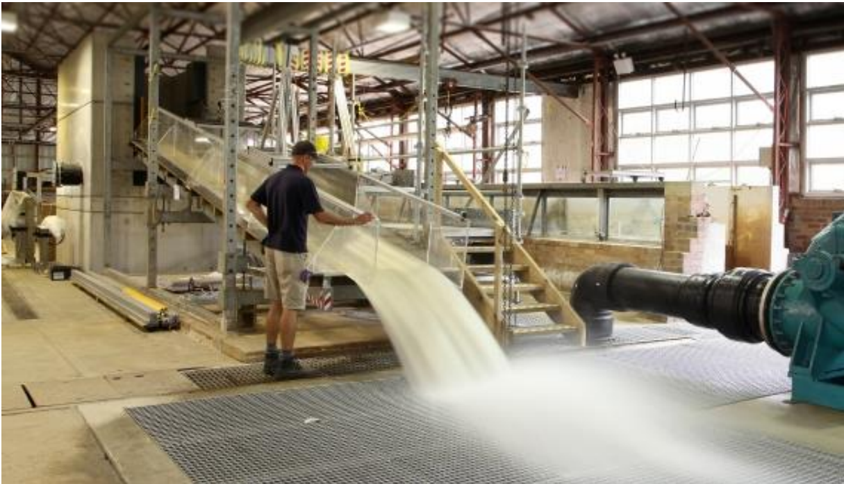
Figure 2-1 WRL spillway flume
