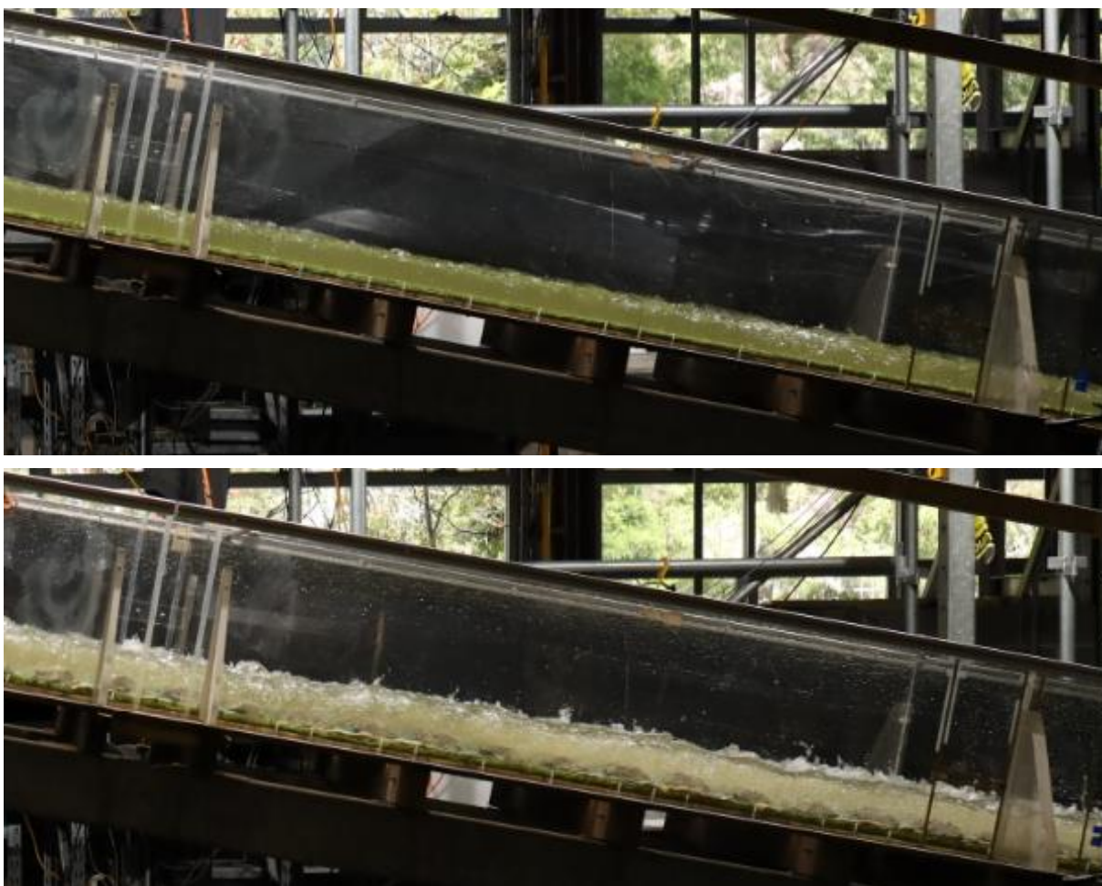
Figure 1-3 Comparison of flows in the artificial turf (top) channel and concrete mattress channel (bottom)
