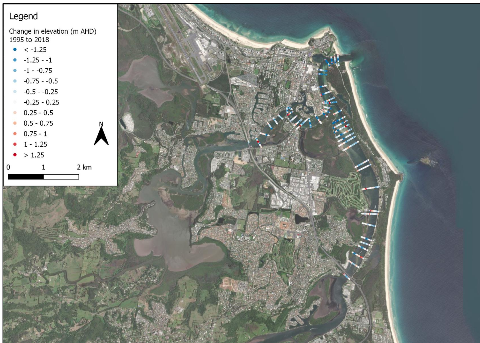
Figure A-1 Bathymetry difference between 1995 survey and 2018 marine LiDAR. Red represents accretion and blue represents erosion
