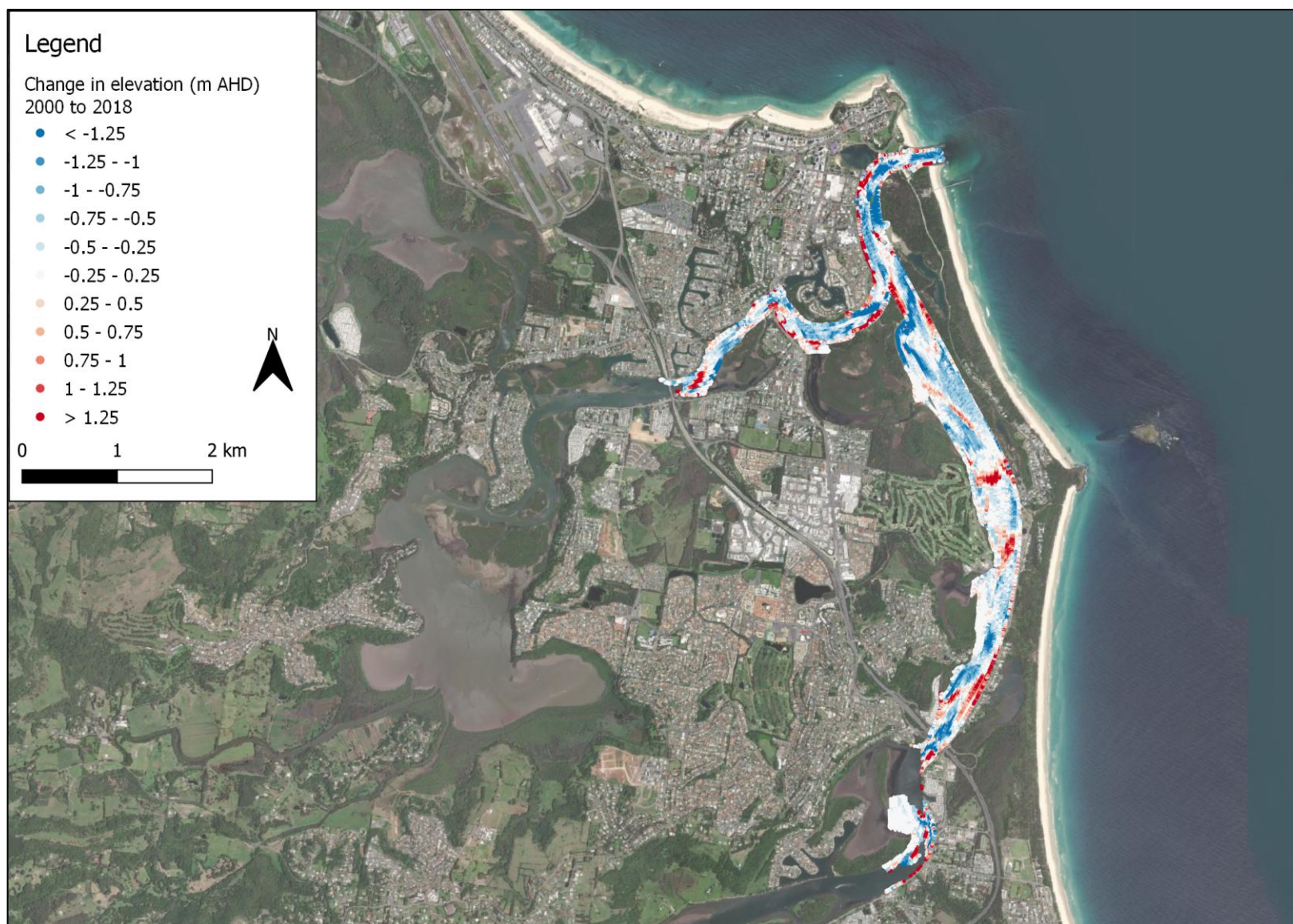
Figure 2-6 Bathymetry difference between 2000 survey and 2018 marine LiDAR. Red represents accretion and blue represents erosion
