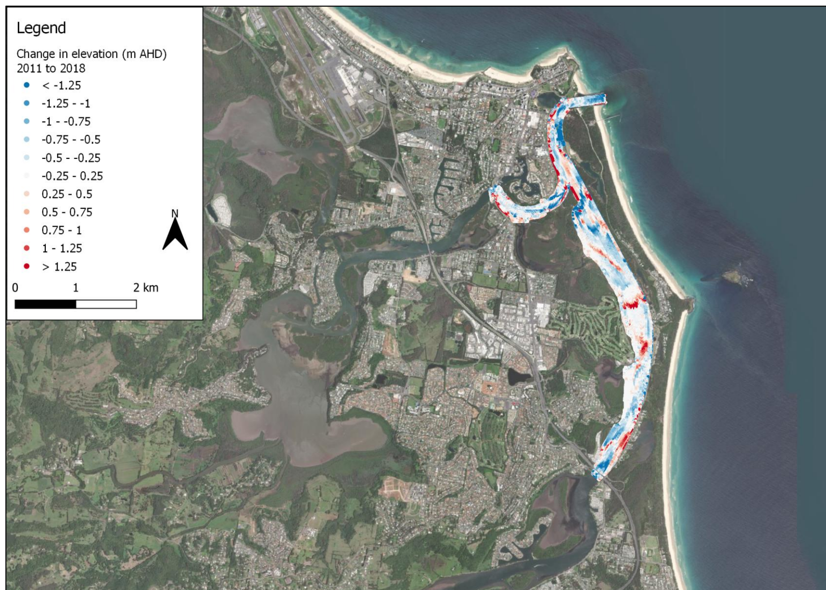
Figure A-3 Bathymetry difference between 2011 survey and 2018 marine LiDAR. Red represents accretion and blue represents erosion
