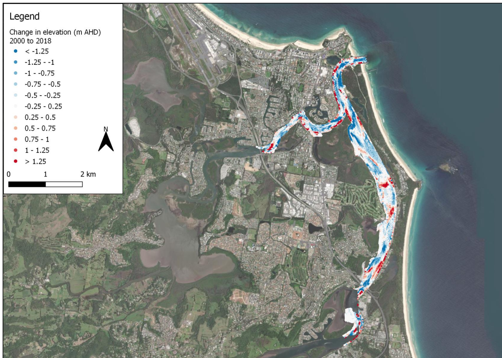
Figure A-2 Bathymetry difference between 2000 survey and 2018 marine LiDAR. Red represents accretion and blue represents erosion
