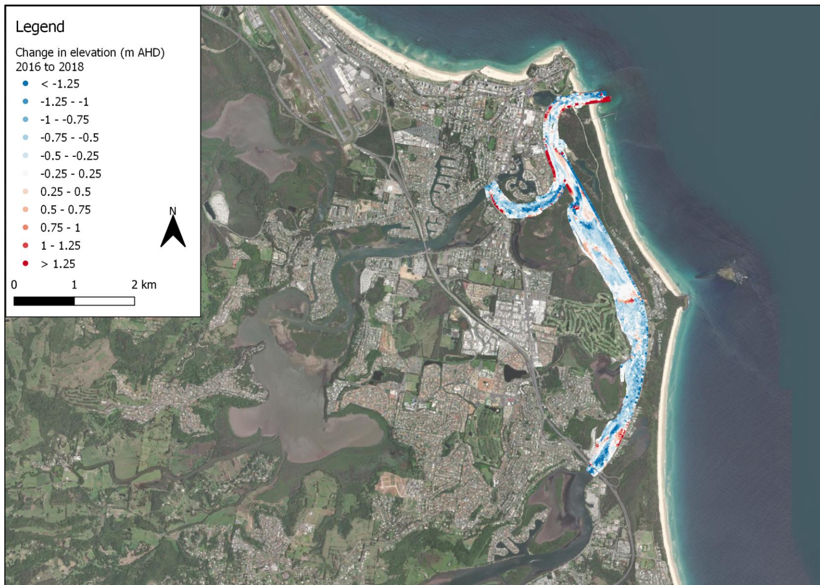
Figure A-5 Bathymetry difference between 2016 survey and 2018 marine LiDAR. Red represents accretion and blue represents erosion
