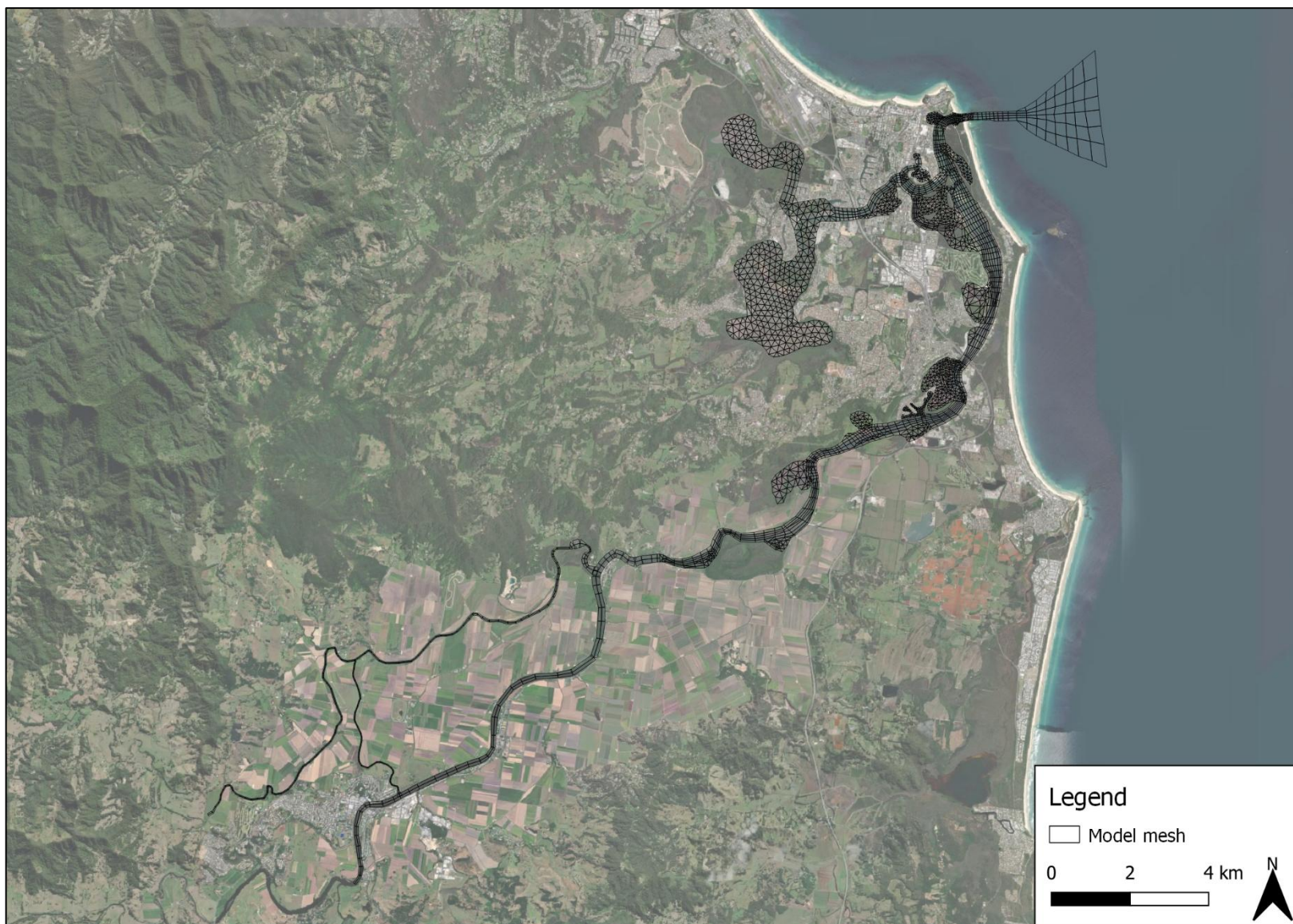
Figure 2-7 Tucker et al. (2023) RMA-2 model mesh geometry extent
