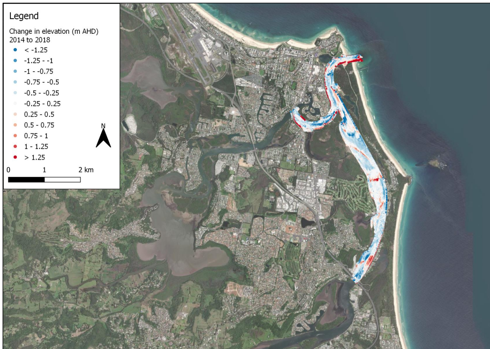
Figure A-4 Bathymetry difference between 2014 survey and 2018 marine LiDAR. Red represents accretion and blue represents erosion
