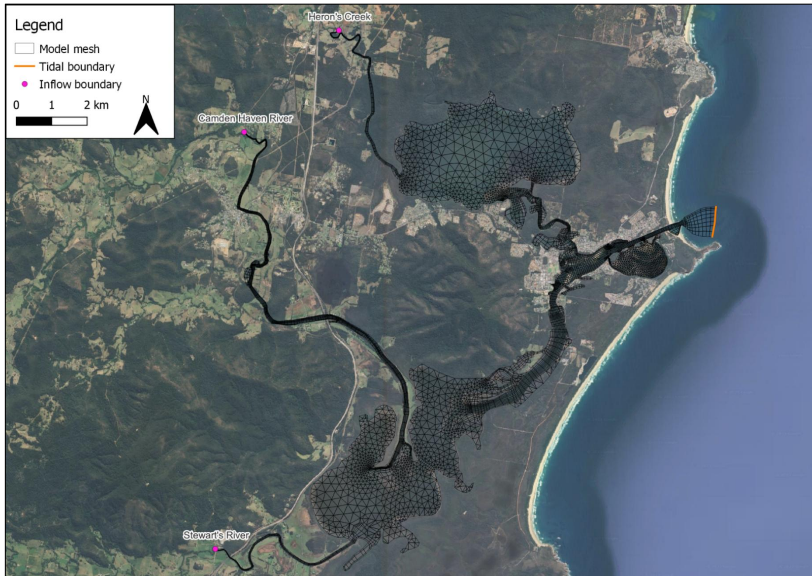
Figure 4-2 RMA model mesh showing boundary condition locations
