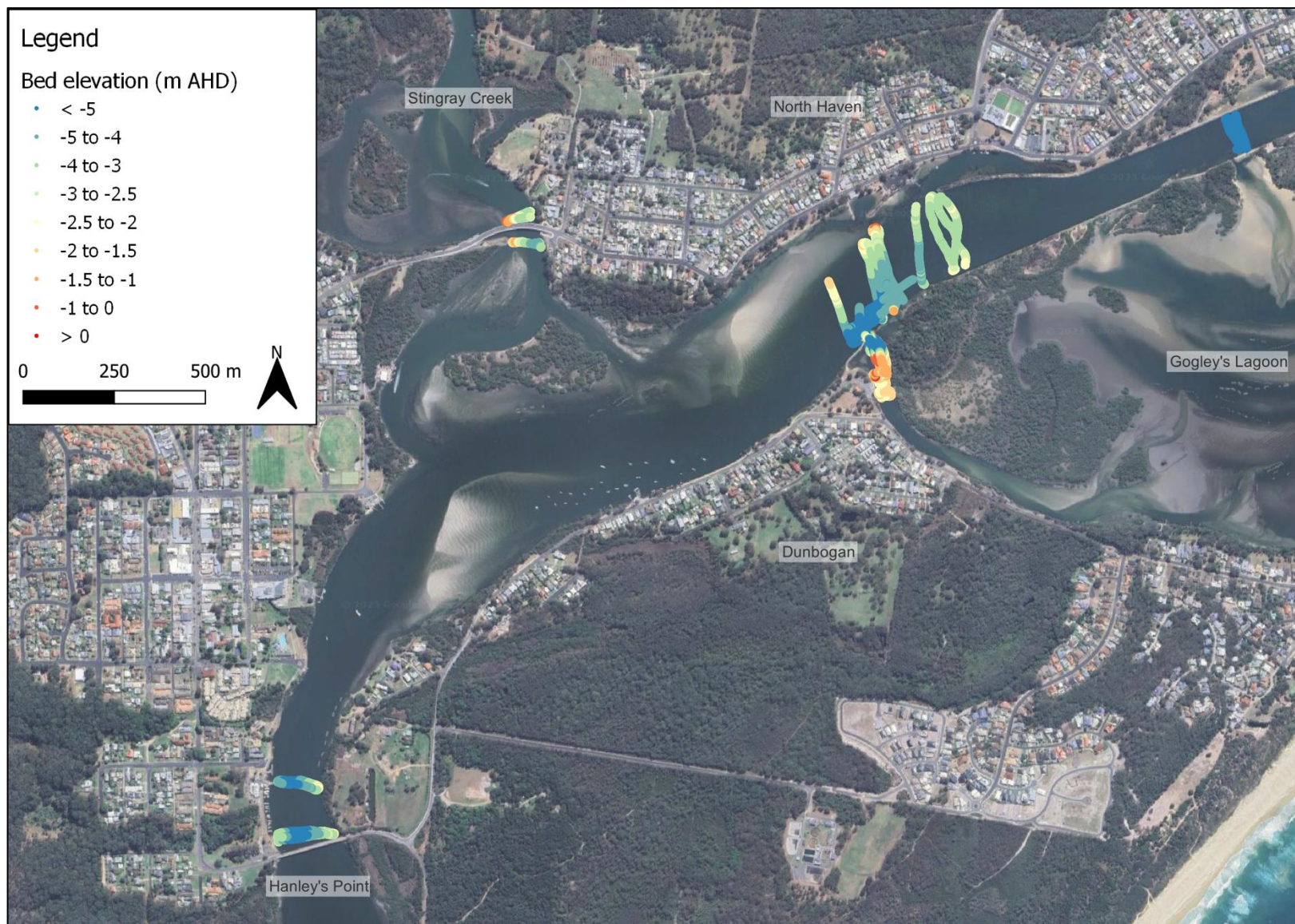
Figure 3-5 Bathymetry collected during 2023 fieldwork
