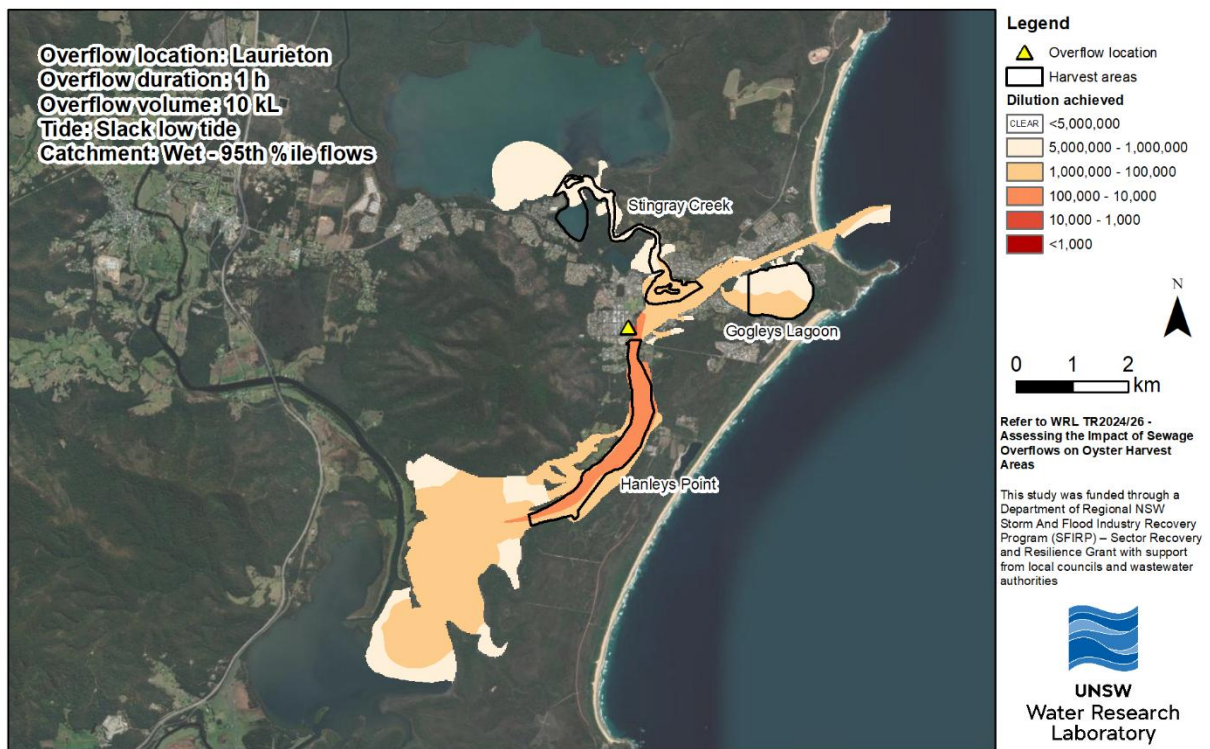
Figure 5-3 Example of a 1-hour overflow at Laurieton during wet (95 th percentile) inflow conditions*
