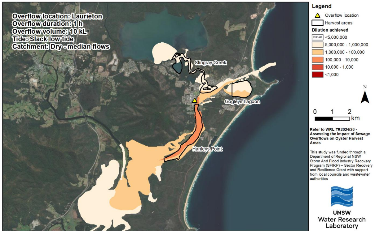
Figure 5-2 Example of a 1-hour overflow at Laurieton during median inflow conditions*
