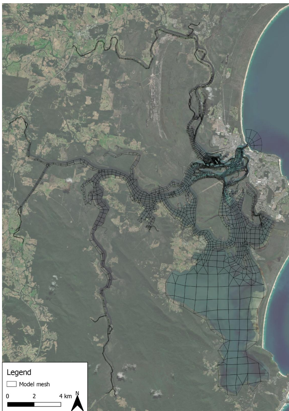
Figure 2-9 Model mesh utilised in WRL TR2006/07
