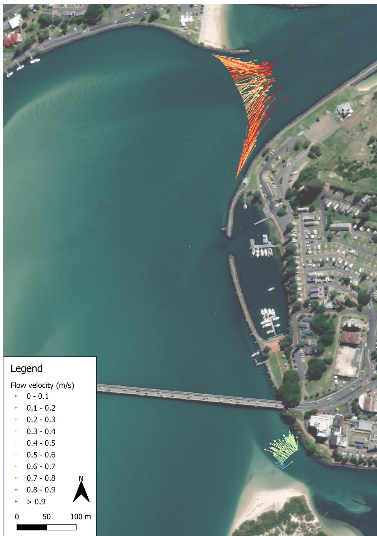
Figure A-10 Ebb tide channel flow distribution at Entrance and Breckenridge
