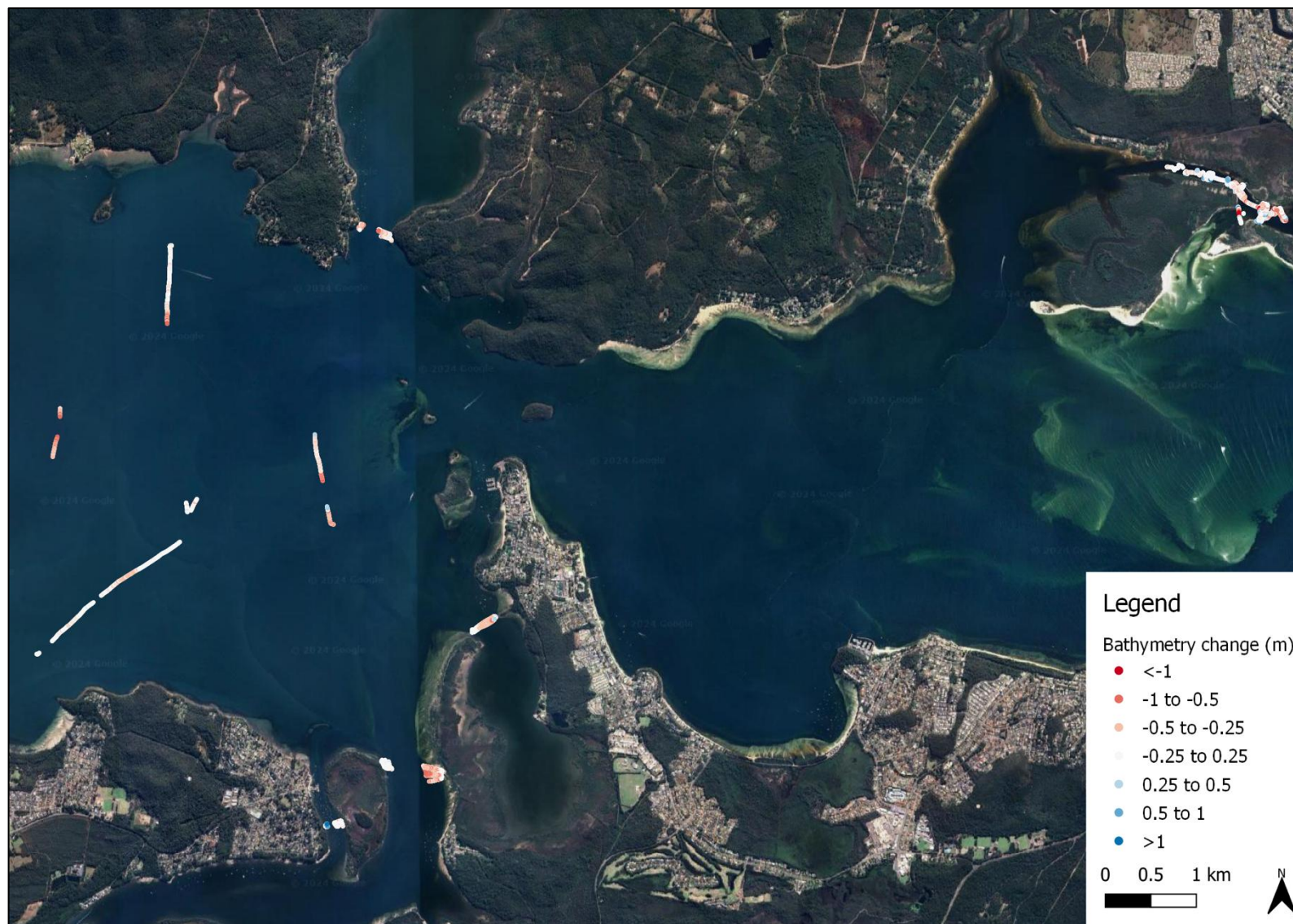
Figure 3-9 Difference between 2018 LiDAR and 2023 fieldwork bathymetry. Red corresponds to erosion and blue to accretion
