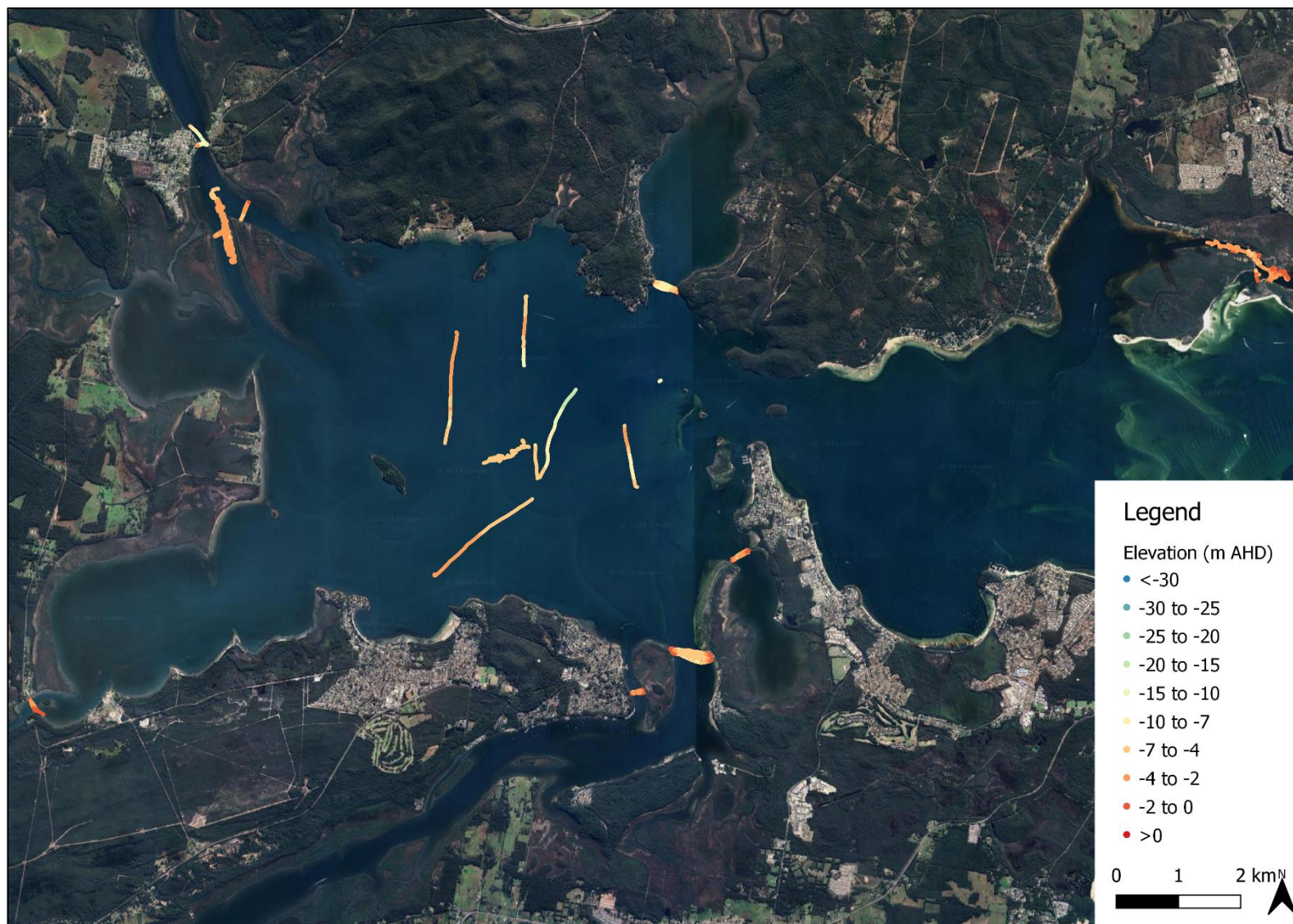
Figure 3-8 Bathymetry collected during 2023 fieldwork
